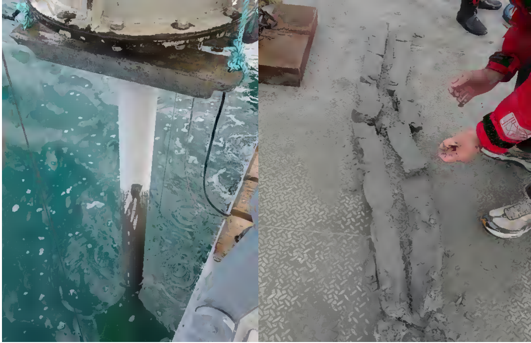
Figure 2-1: Sediment core being retrieved at the side of the vessel showing soft sediment on the outer core (left). A core from the upper Kenepuru that extruded on the vessel deck after failure of the 'core-catcher'. The top of the core is in the foreground (right).
