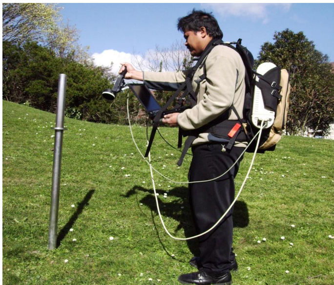
Fig.13 Backpack Vis-NIR DRS apparatus for field collection of soil spectra. The backpack contains three spectrophotometers which receive hyperspectral reflective energy via a fibre optic cable from the soil surface. Note the prototype soil probe developed to collect soil spectra (being held by B. Kusumo), and the soil corer used to extract soil cores.
