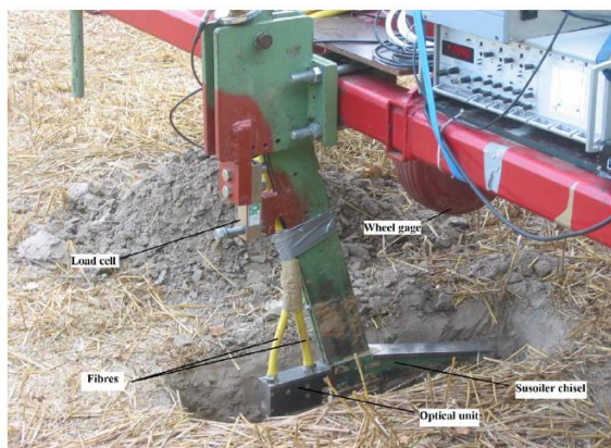
Fig. 10 Subsoiler-optical unit for on-line Vis-NIR DRS field measurement (Mouazen et al. 2005).
