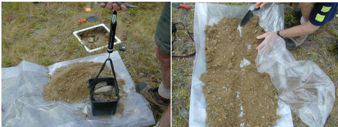
Fig. 5 An example of weighing gravel (left) and sub-sampling during quantitative pit excavation (right) (after Davis et al. 2004).
