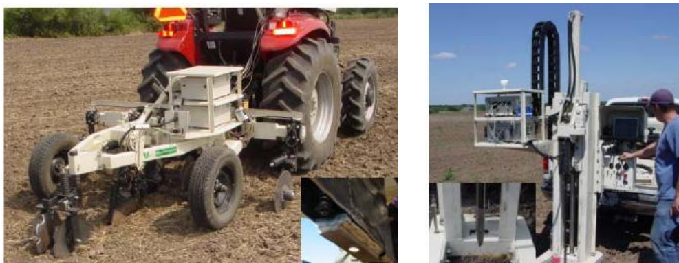
Fig. 11 Vis-NIR DRS shank module (left) and the Vis-NIR DRS probe module (right) (Lund et al. 2008).
