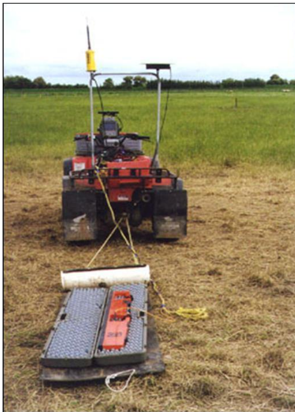
Fig. 16 On-the-go EM mapping system, employing a Geonics EM38, RTK-GPS, datalogger, on-board field computer and ATV
