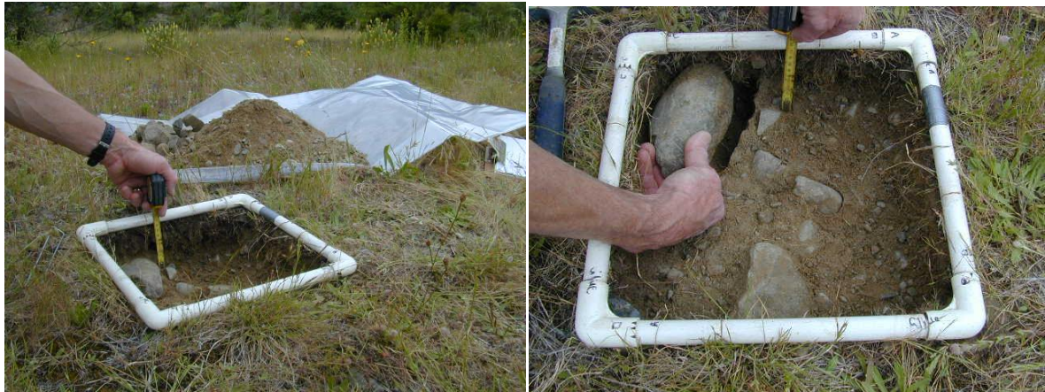
Fig. 4 An example of the excavation of a quantitative pit to 0.1 m depth in a soil containing coarse gravel (after Davis et al. 2004).
