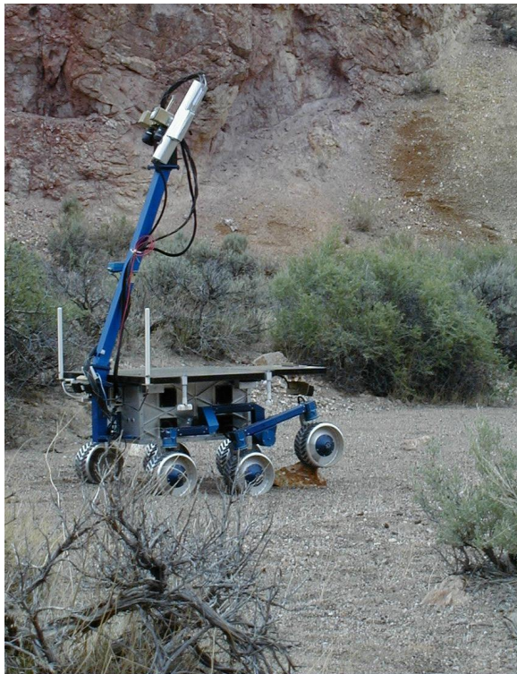
Fig. 20 NASA AMES K-9 rover fitted with prototype LIBS instrument, with the laser and telescope on the mast and spectrograph, detector and electronics in the body (Image from NASA Ames Research Centre).
