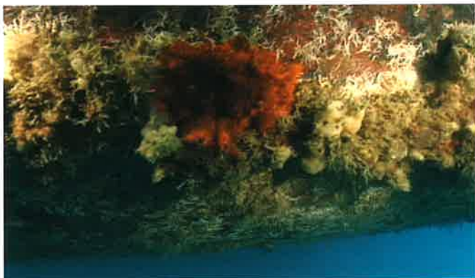
Fouling on the hull of an overseas yacht.
