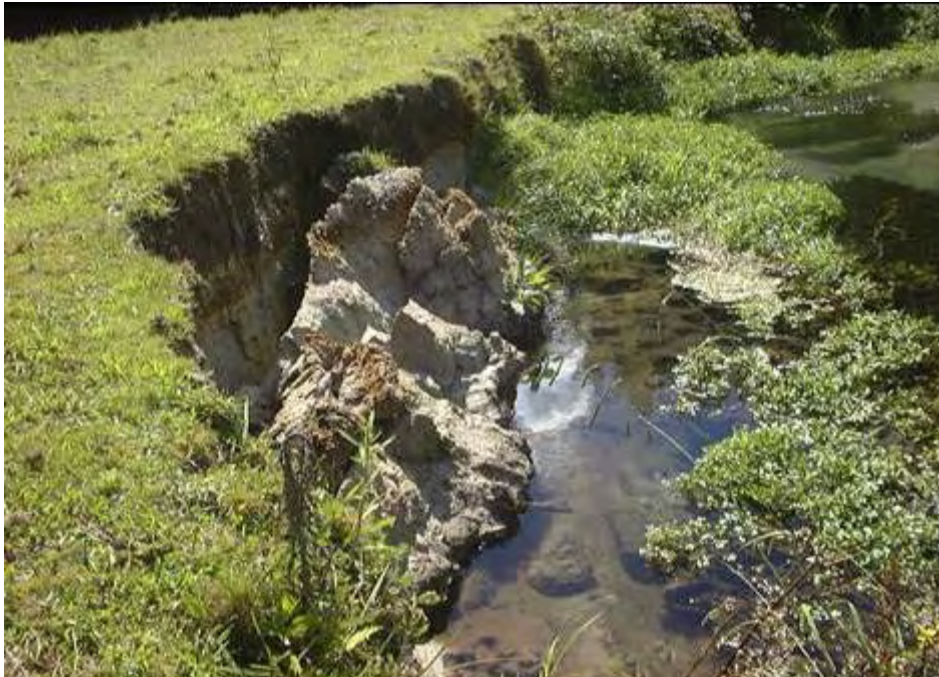
Figure 20: An example of slump erosion; coding and description. SI (A) o 6 x 1.5 m N: Slump, (active), outside, 6 m long, 1.5 m high, not protected.
