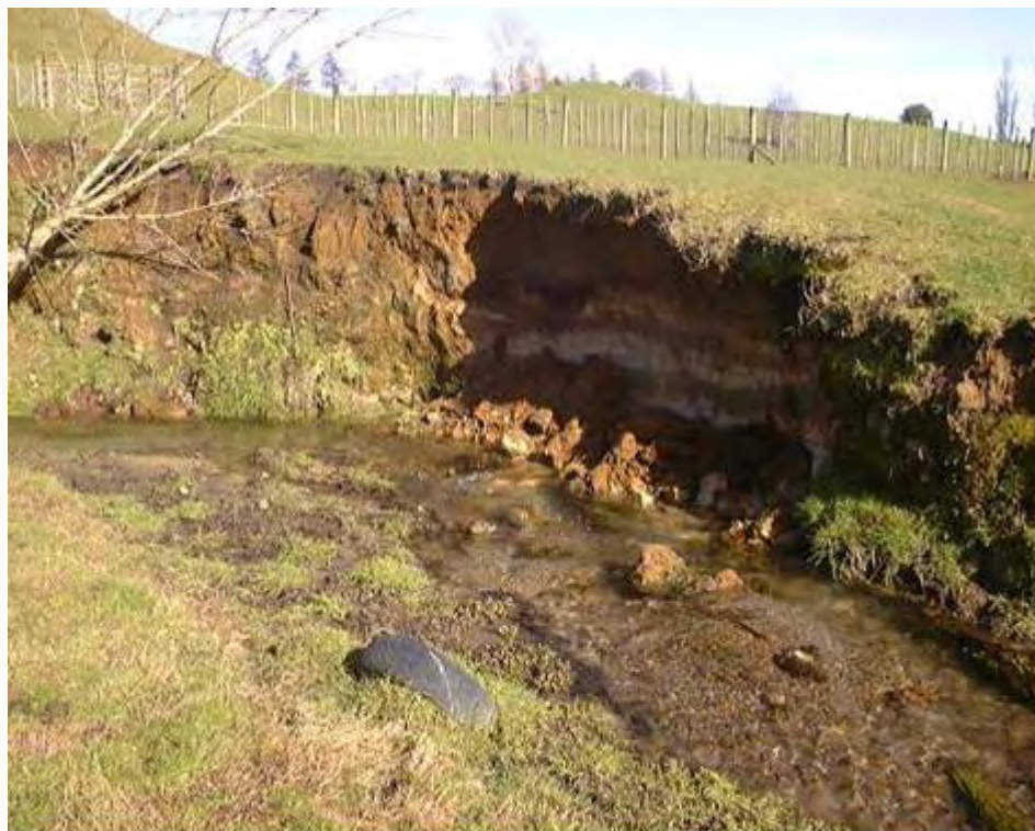
Figure 19: An example of slump erosion; coding and description. Sm (A) o 5 x 2 N: Slump, (active), outside, 5 m long, 2 m high, not protected. Note that the active section of erosion recorded separate to unstable section of erosion.
