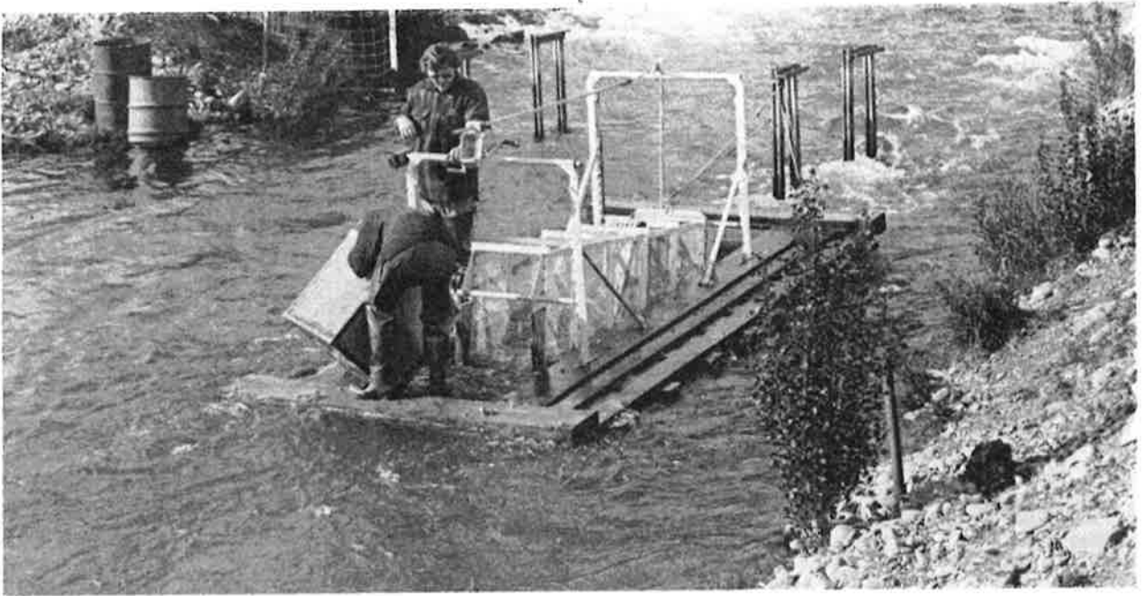
A floating fry trap below the main Glenariffe trap. The fry trap has been used to estimate losses of fry and juveniles from the system as well as to provide additional information on migration of smolts.
