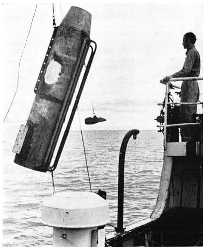
Collections of planktonic fish eggs and larvae are used for identification of spawning areas and spawning seasons as well as for estimating fish abundance. A "tin-tow net" or high-speed plankton sampler, which is shown being lowered over the side of the research vessel James Cook , is often used for the purpose.
