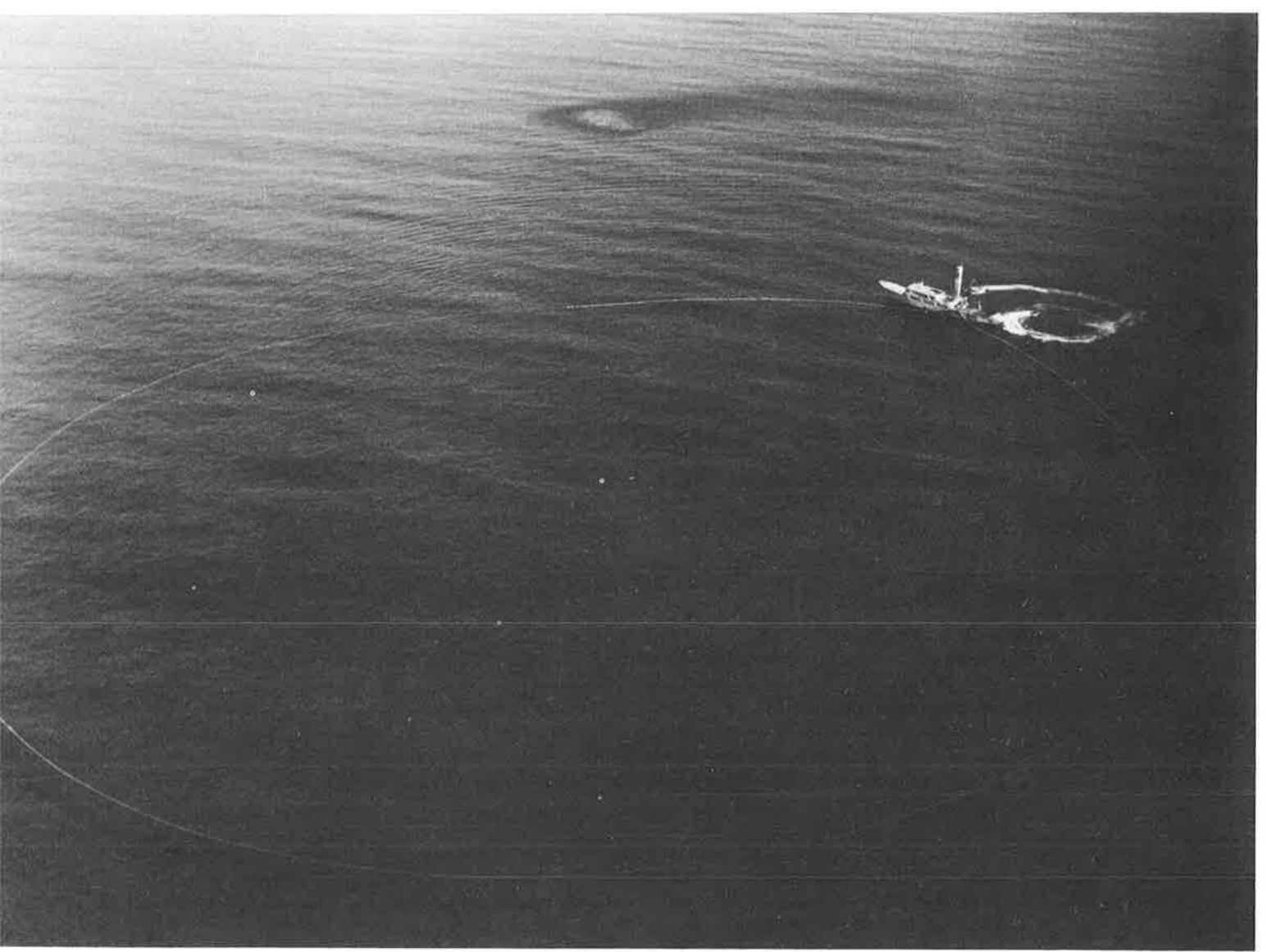
A joint venture purse-seine vessel in set. Note the circling skiff and speedboat near the vessel and the large (over 100-t) school of skipjack outside the net.
