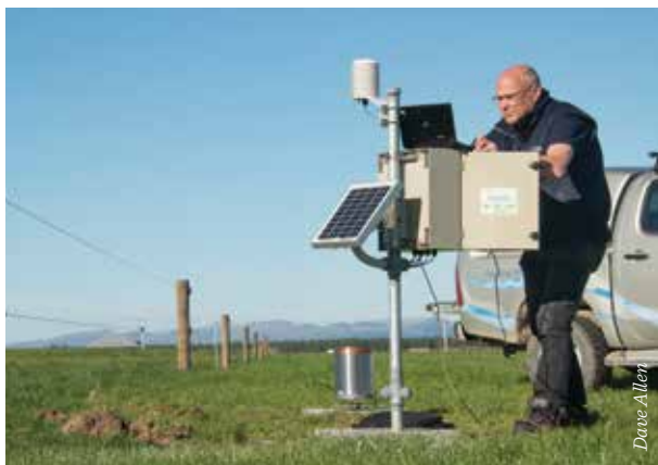
An IrriMet monitoring station in Canterbury, feeding weather and soil-moisture data direct to NIWA's supercomputer in Wellington. Information is sent back to the farmer, via the internet, in the form of simple guidance on when – and when not – to irrigate or fertilise.
