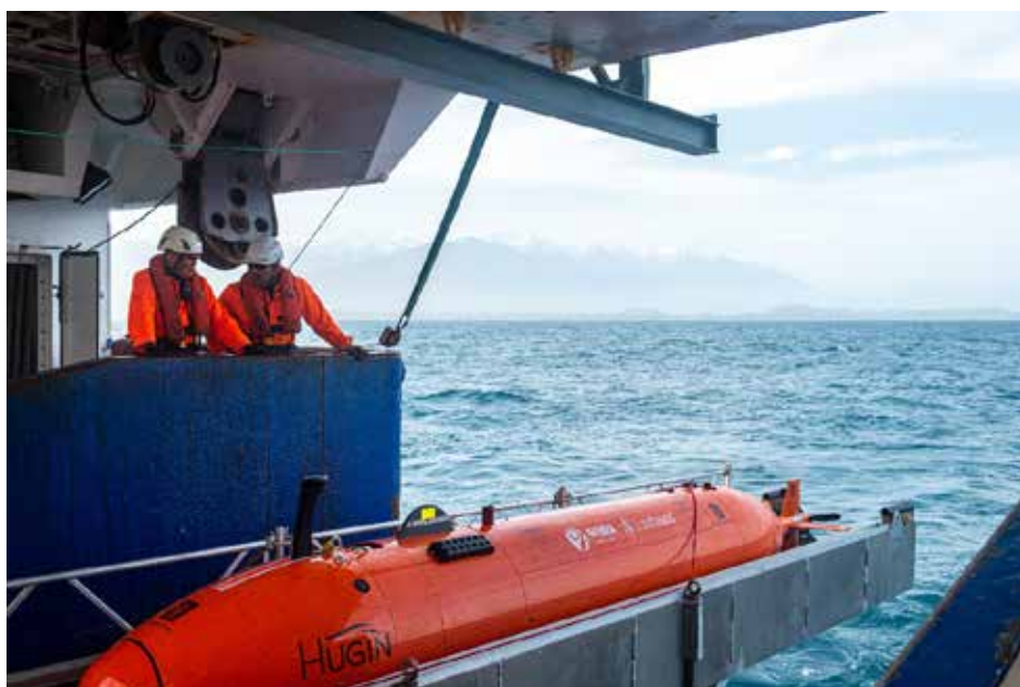
NIWA marine geologists collaborated with Swedish colleagues from the University of Gothenburg to bring this 6.5m autonomous underwater vehicle (AUV) to New Zealand for deployment off Tangaroa for detailed bathymetric mapping of the Kaikoura Canyon seafloor. [Lana Young]
