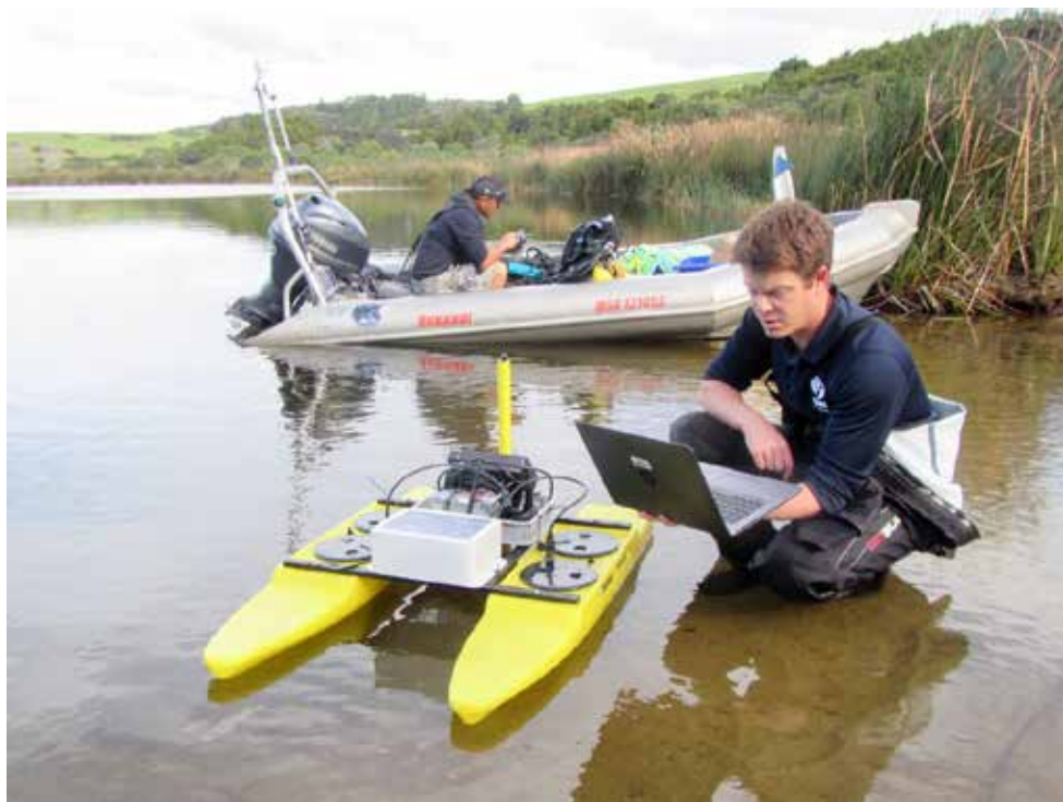
NIWA freshwater scientists trialling new technologies combining Artificial Intelligence (AI) software with autonomous boats to detect invasive weeds in Waikato waterways. [Mary De Winton]
