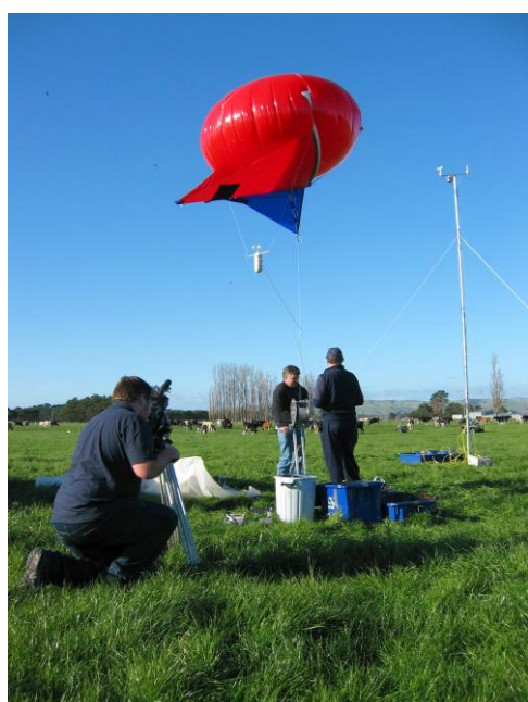
Figure 3. Helikite being raised with suspended radiosonde and sampling tubes at various heights
