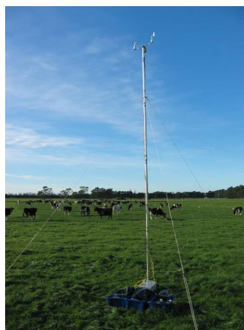
Figure 4. Fixed 6-m mast with anemometer and sample collection tubes at various heights
