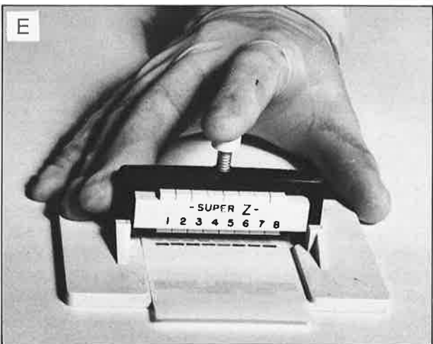
Figure 4: Preparation of cellulose acetate gels for electrophoresis. A, placing electrode wicks into the electrode tank; B, adding the plates to the gel buffer; C, pouring the gel buffer into the header tank to soak the plates in the lower chamber; D, adding supernatant to the loading base; E, printing samples on the gel; F, putting the gel plates into the electrophoretic tank.
