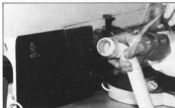
Figure 14: Drying an agarose gel (on a gel backing sheet) with a hairdryer.
