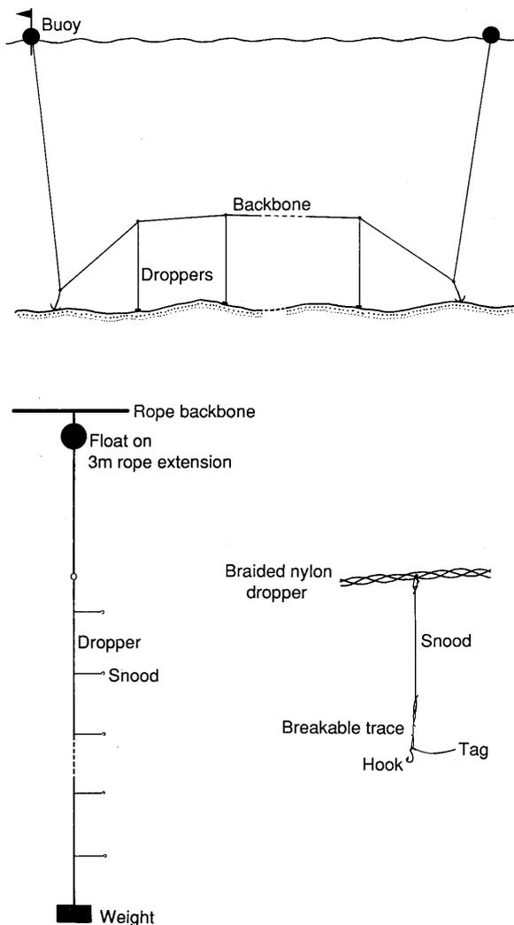
Figure 2: Fishing gear configuration used during the pilot survey and the detachable tagging survey.
