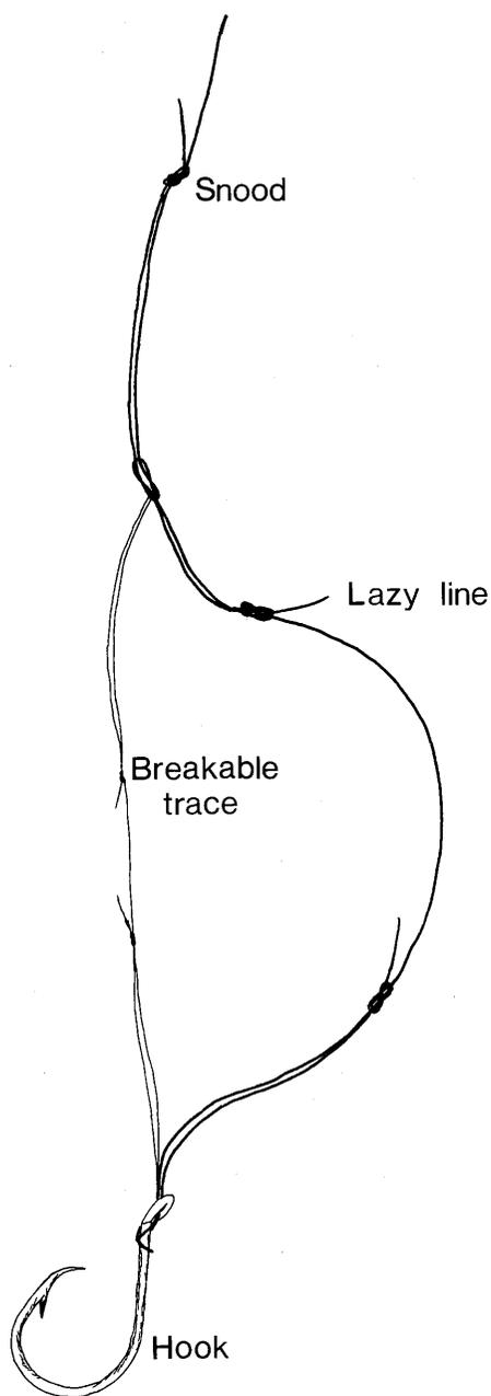
Figure 5: Snood and breakable trace with full strength lazy line. (Fish capable of breaking the weak trace are still retained on this gear.)
