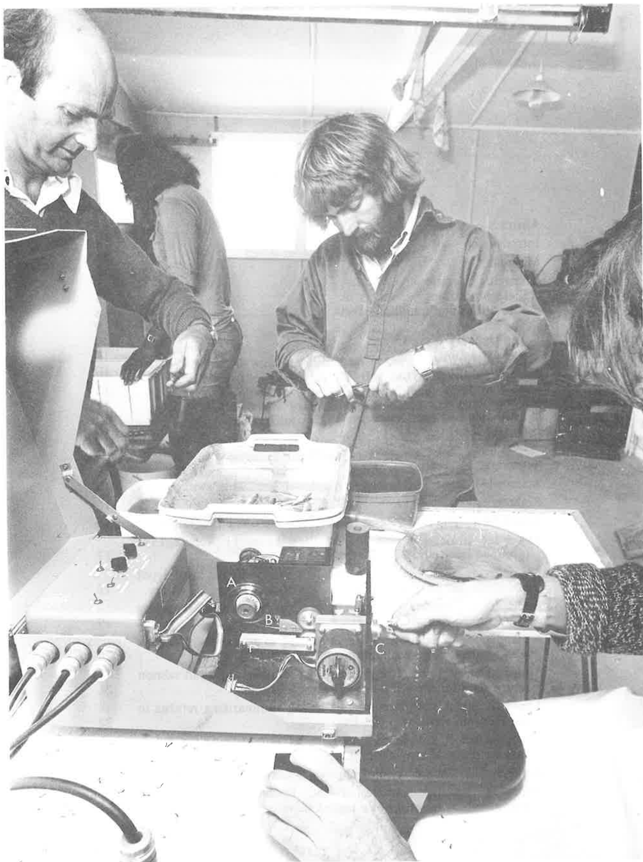
Salmon tagging at FFC's Glenariffe hatchery, January 1979. Clearly visible inside the tagging machine are the spool of pre-coded tagging wire (A) and a length of this wire (B) feeding into the injection unit. A tranquillised salmon is about to be inserted into the head mould (C), while the operator controls the machine with a button under his left hand. Two assistants are removing adipose fins from the fish (before tagging), while the fourth member of the crew (background) is transferring fish to and from the tranquilliser baths as required. (Photograph courtesy Christchurch Star .)
