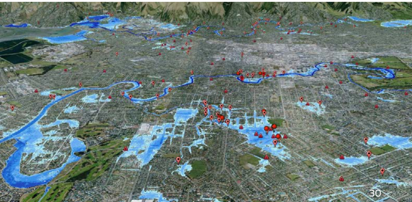
Christchurch under water: flooded areas shown in blue; emergency callouts and field measurement locations also shown. Note the darker the blue, the greater the flooding. Data: NIWA.
