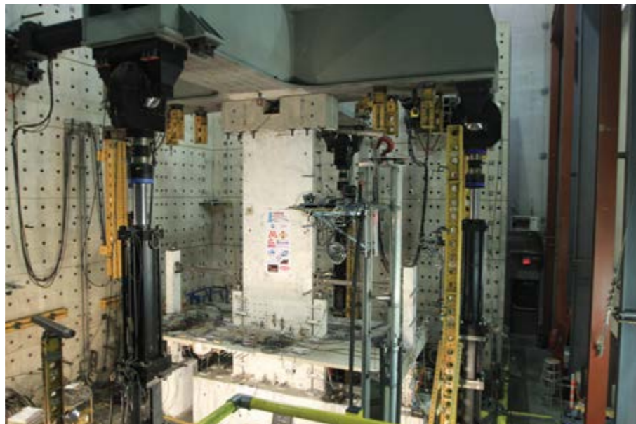
Figure 3. Low-damage rocking wall system test at the University of Minnesota.
