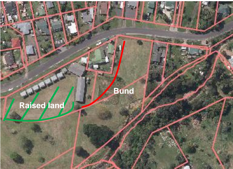
Figure 24 Indicative alignment for bund/flood wall
