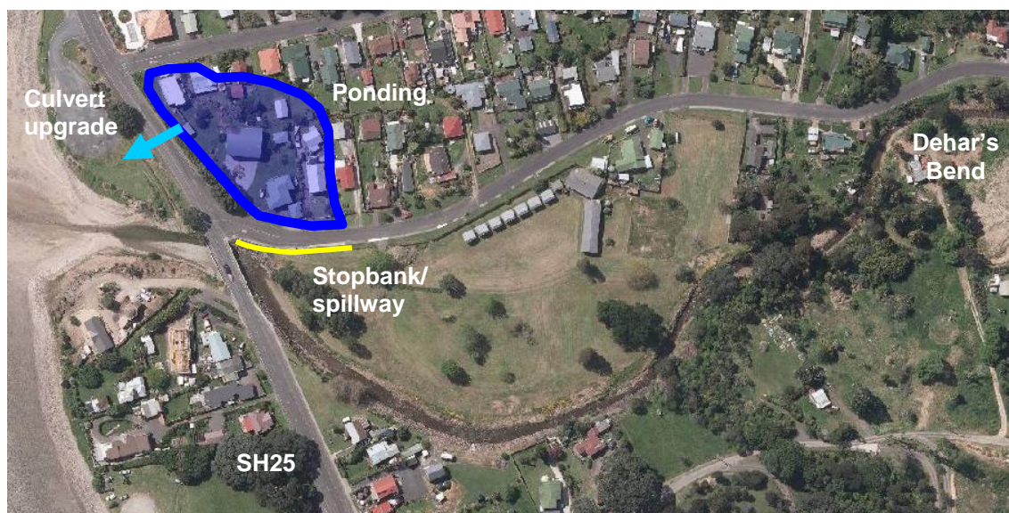
Figure 27 Proposed culvert upgrade
