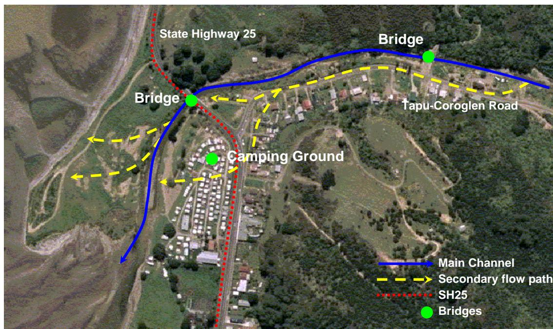
**Figure 6 Predominant flooding mechanism at Tapu during a significant flood event**
