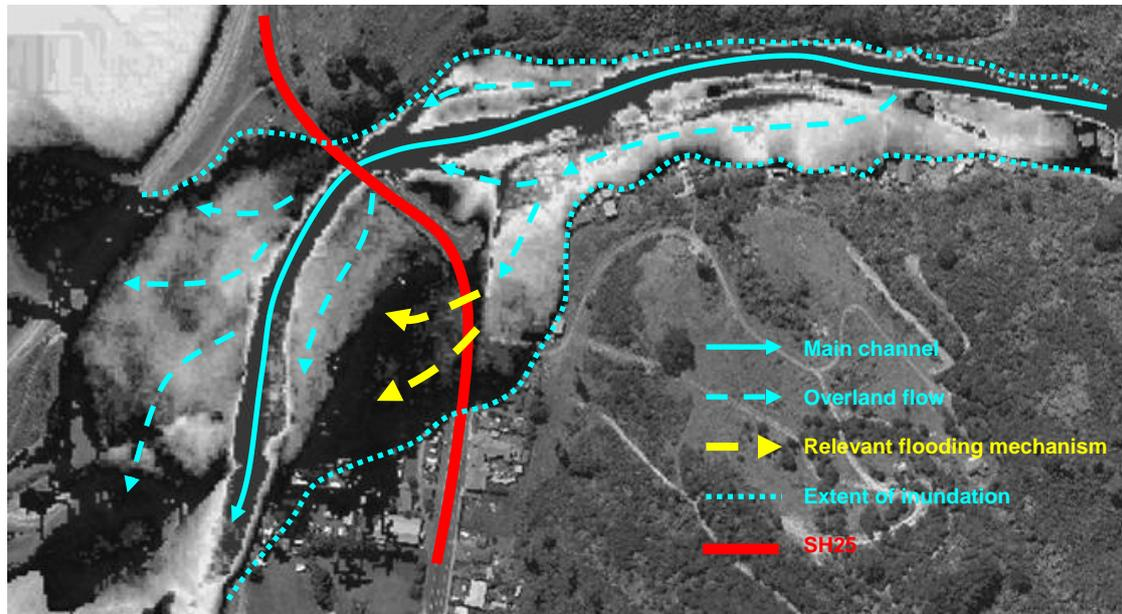
**Figure 14 Flooding mechanisms relevant to spillway design**
