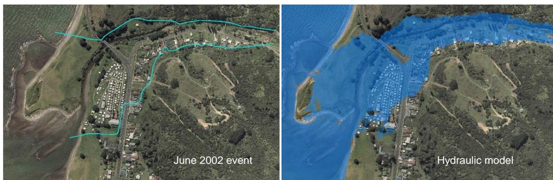
Figure 11 Comparison of modelled and observed flood extents
