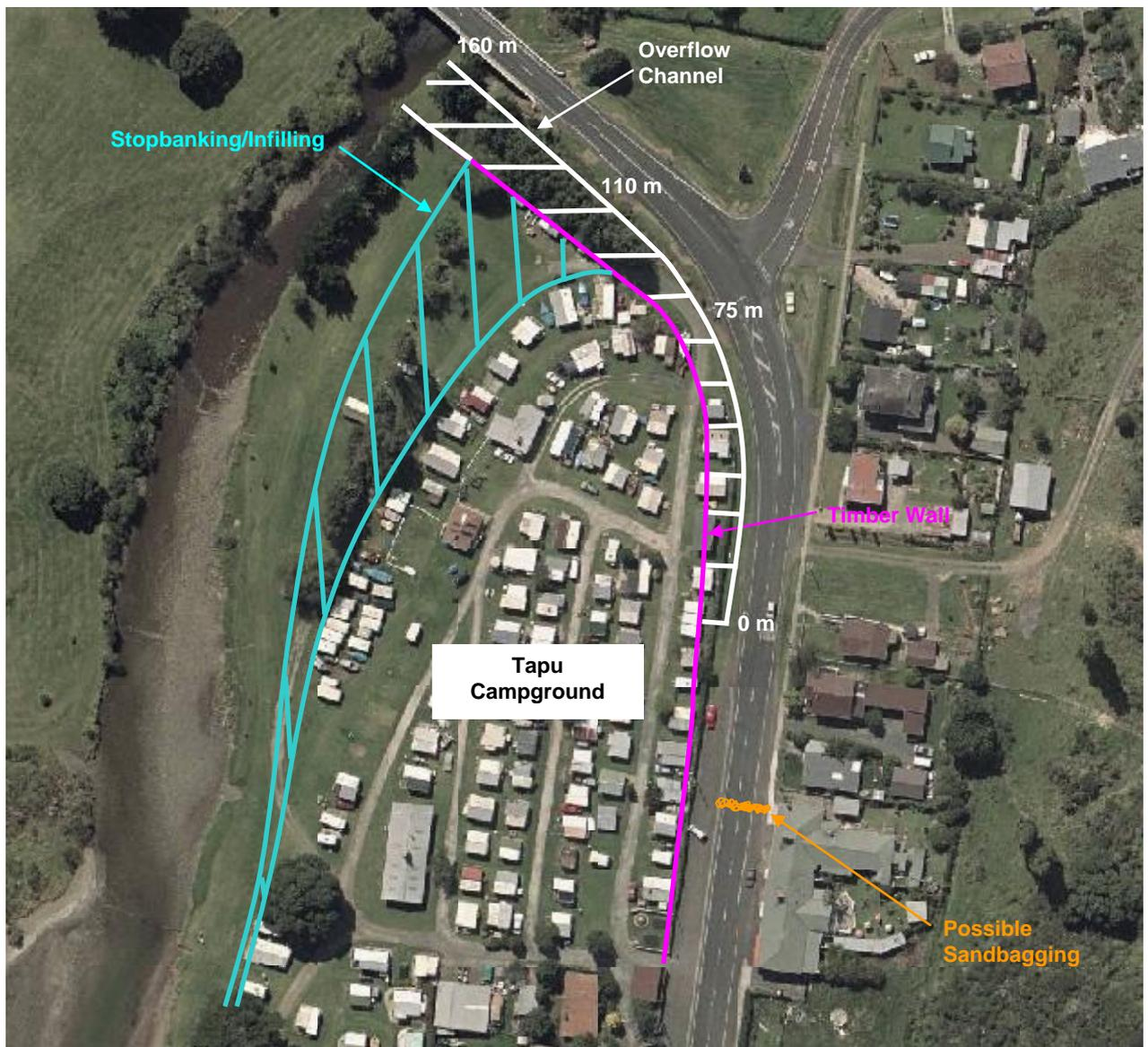
**Figure 13 Flood protection scheme**
