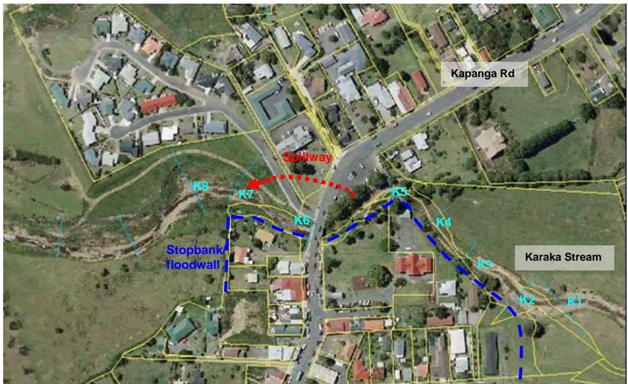
Figure 20 Flood defence constructed at Kapanga Road bridge
