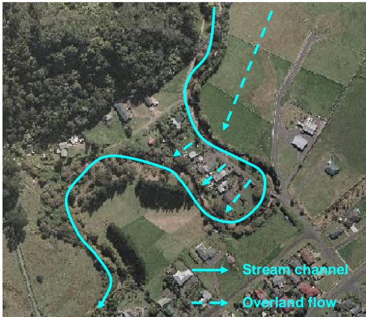
Figure 17 Overland flow across the Albert Street meander during significant flood events
