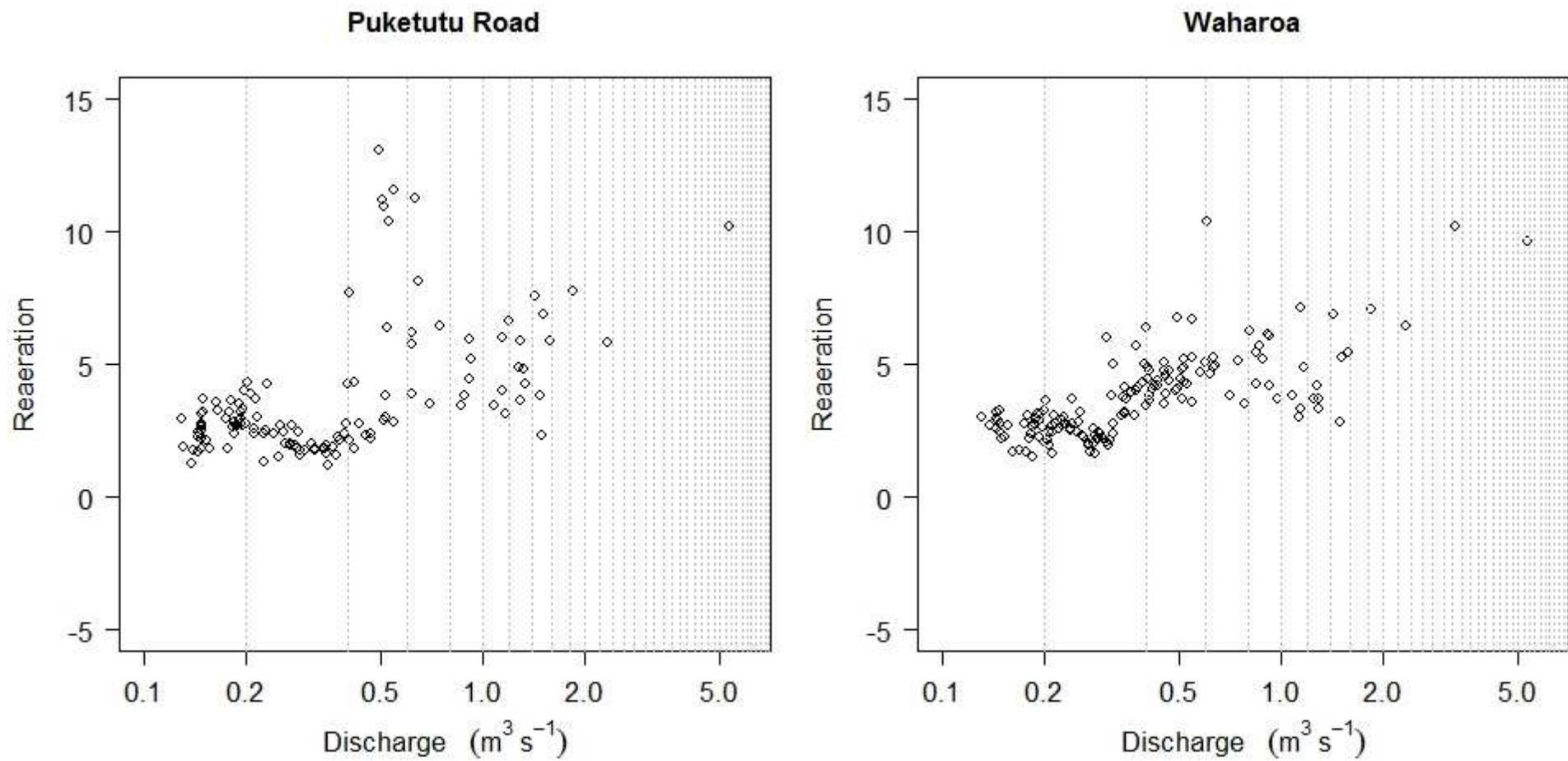
Figure 3-20: Scatter plots of the estimated reaeration coefficient ( $k_2$ ) and river flow at the Puketutu Road and Waharoa sampling sites on the Waitoa River.
