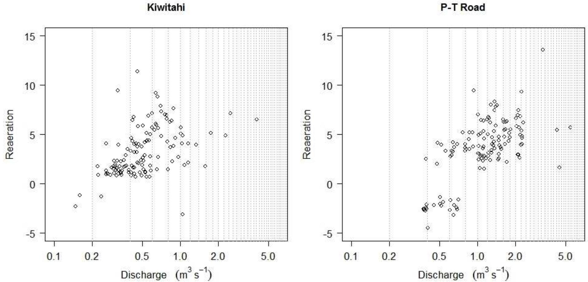
Figure 3-19: Scatter plots of the estimated reaeration coefficient ( $k_2$ ) and river flow at the Kiwitahi and Paeroa-Tahuna Road sampling sites on the Piako River.
