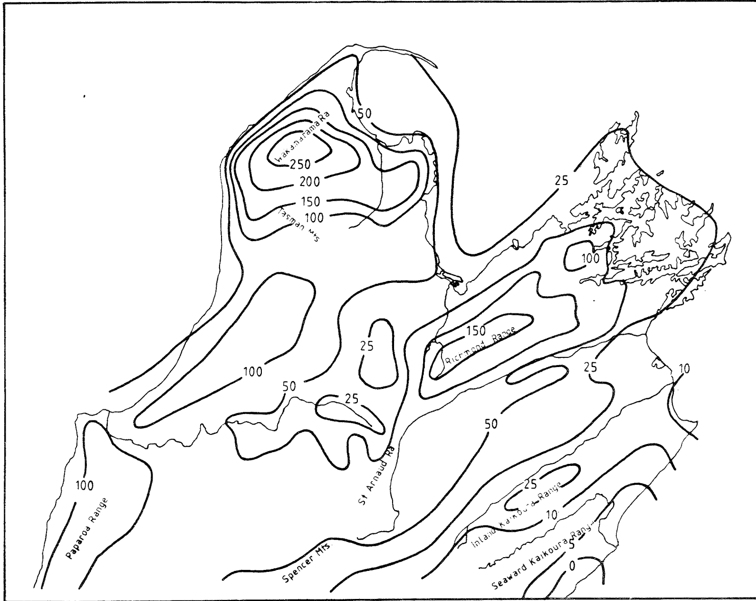
Fig. 6: Isohyets (mm) of 24 hour rainfall, 8 July 1983. (9am July 8th to 9am July 9th).
