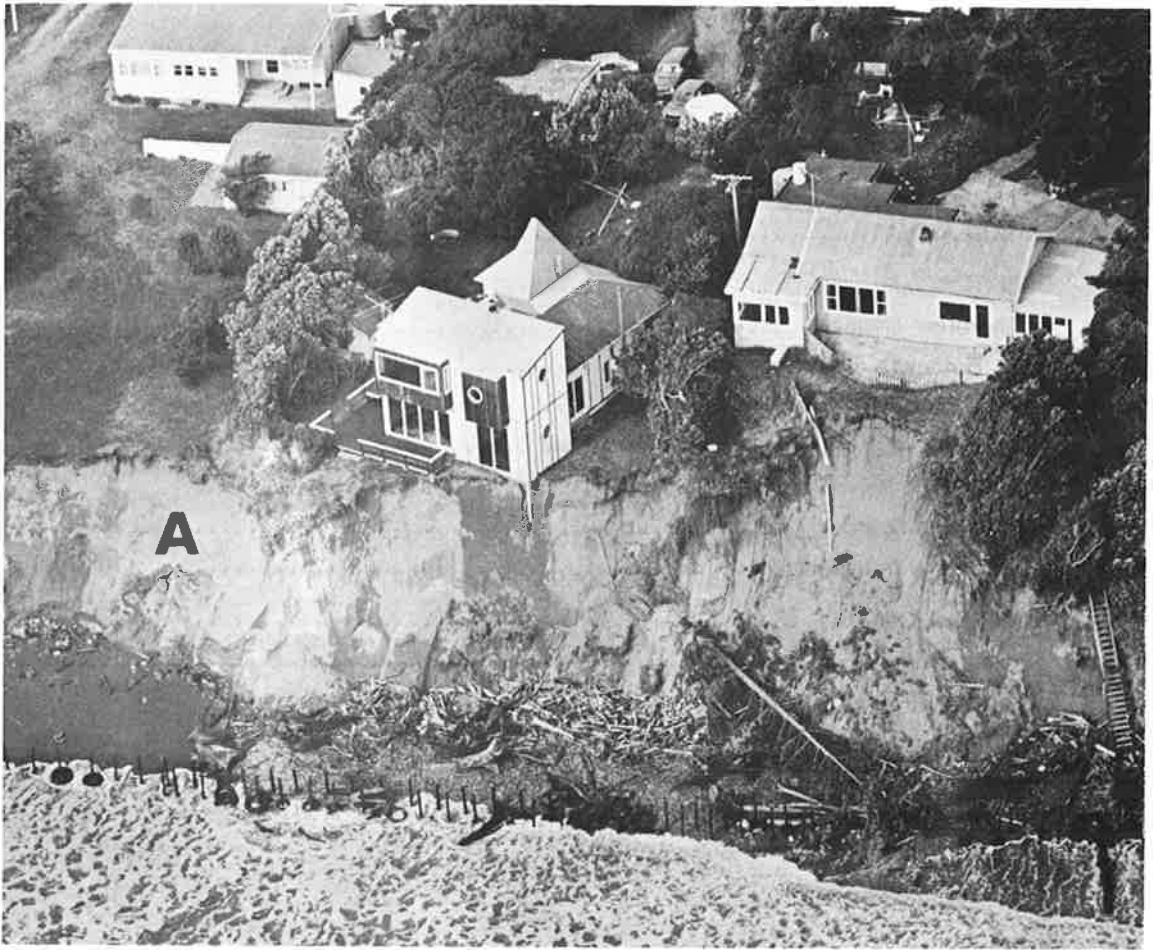
FIG. 1 Coastal erosion and protection at Raumati Beach, 'Golden Coast'.
