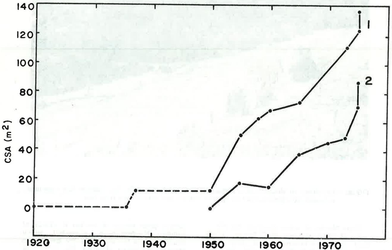
FIG 11 – Cumulative decreases of channel cross-sectional area (CSA) resulting from deposition of alluvium on McCullough's mill reach for: 1. section C, 2. average of sections A-C (1955-60) and A-F (1960-75).
