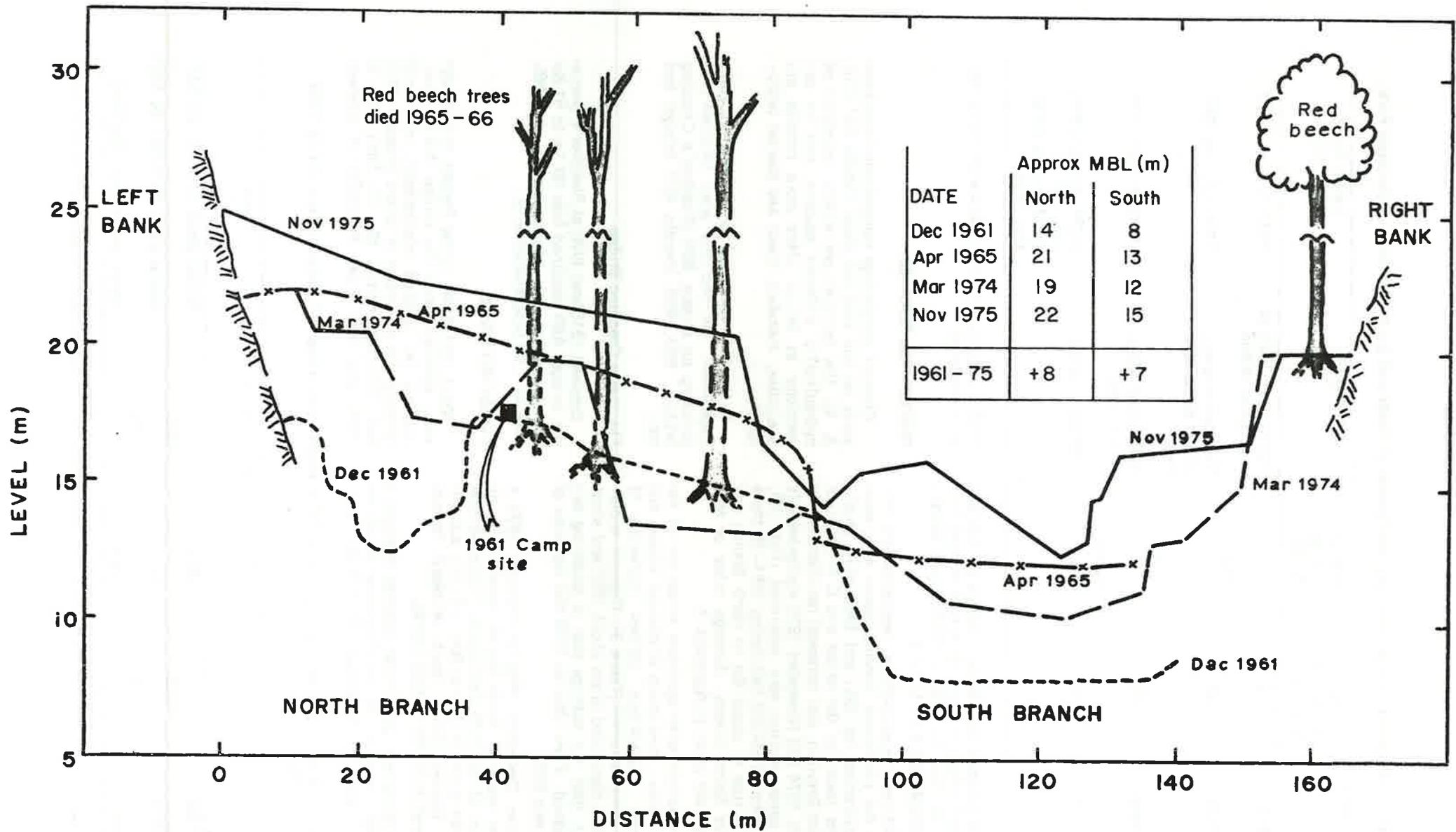
FIG 14 - Channel profiles at the Waipawa Fork section.
