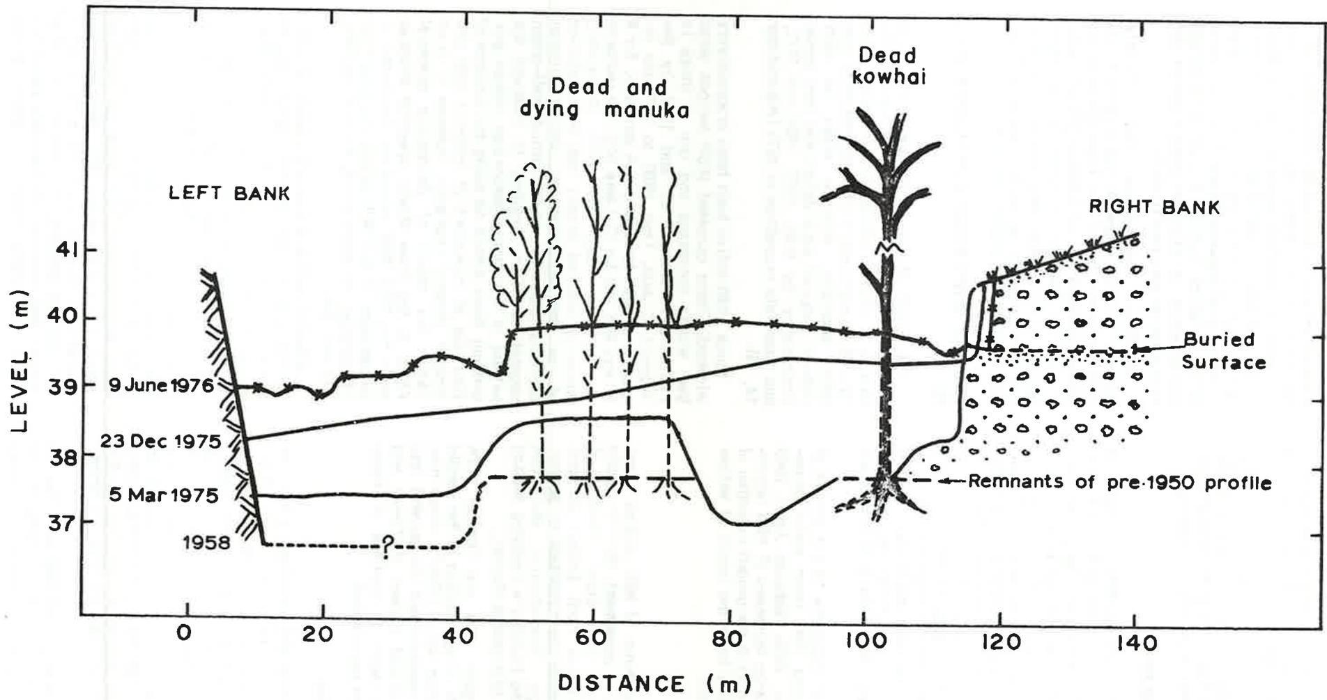
FIG 15 – Channel profiles at the kowhai section.
