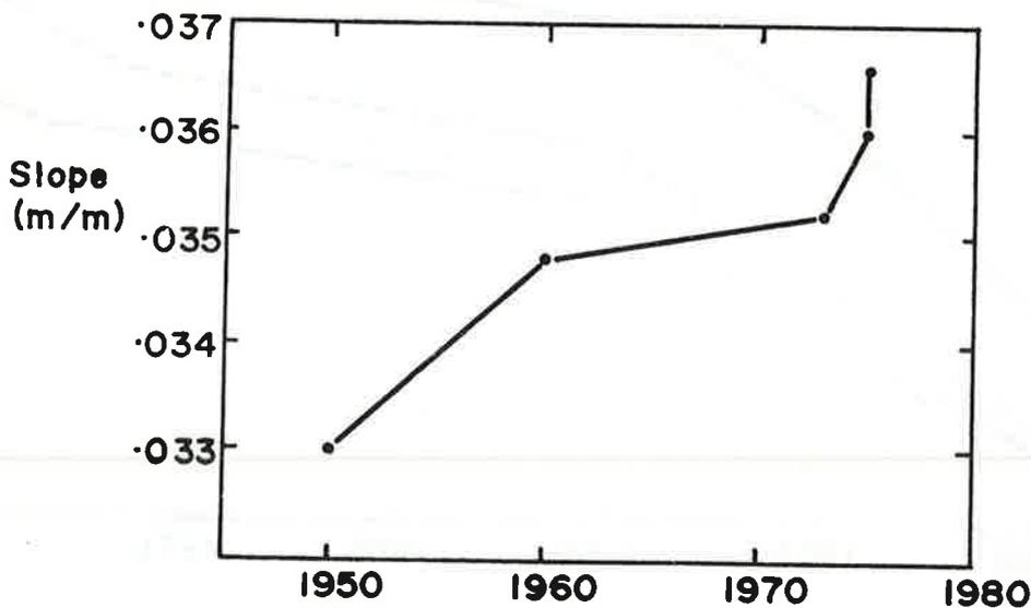
FIG 8 – Changes of mean channel slope on McCullough’s mill reach.
