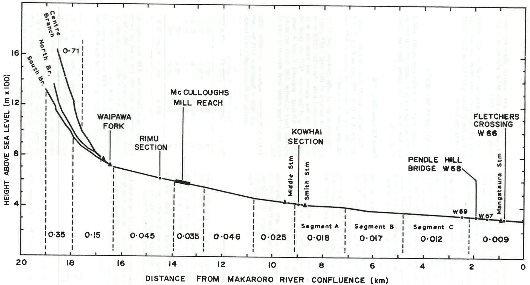
FIG 4 - Channel longitudinal profile of the upper Waipawa River. Approximate average slope values are shown.
