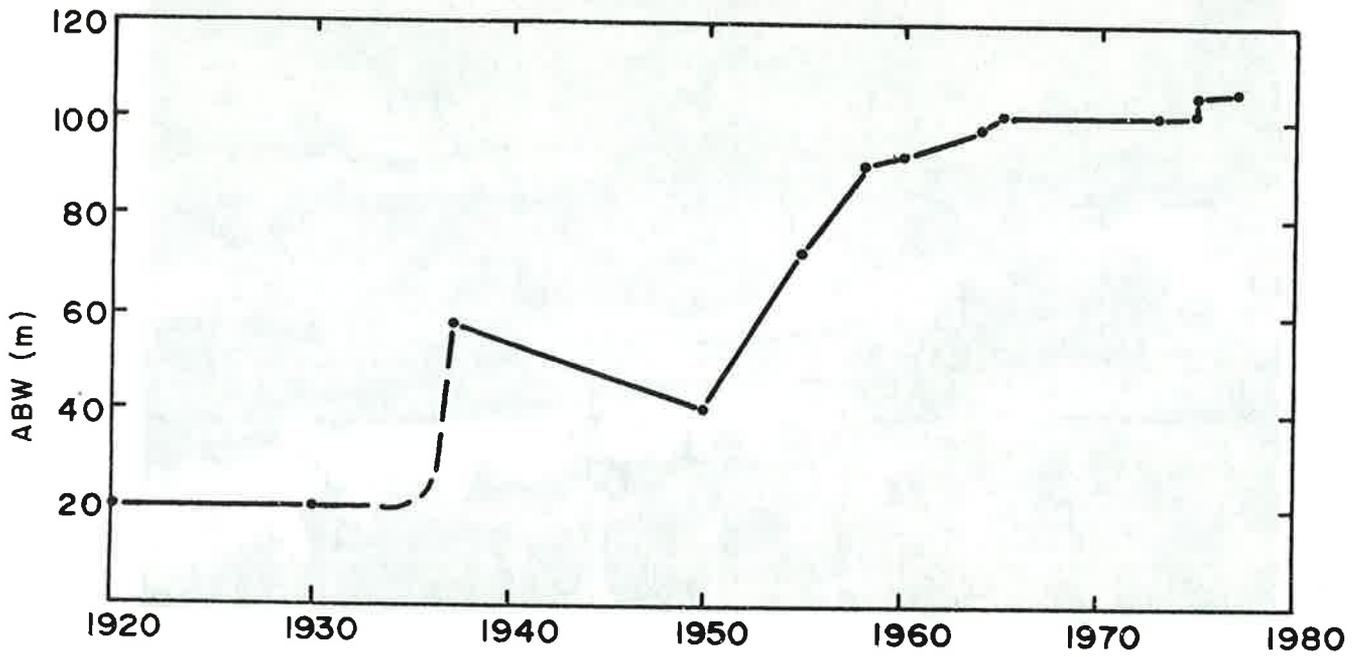
FIG 10 – Changes of ABW at section C on McCullough's mill reach.
