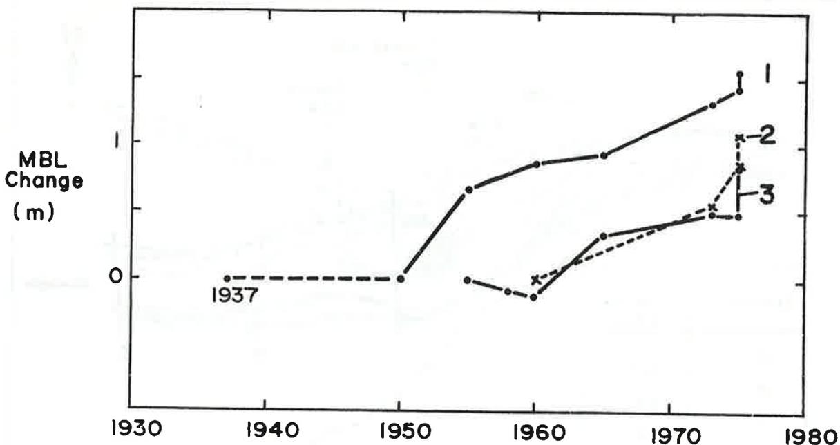
FIG 7 – Cumulative changes of MBL on McCullough’s mill reach for : 1. section C, 2. sections A–F, 3. sections A–C.
