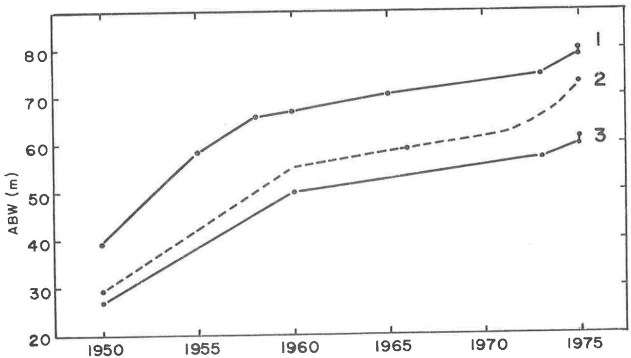
FIG 6 – Changes of average ABW on McCullough's mill reach based on : 1. sections A-C, 2. aerial photos, 3. sections A-F.
