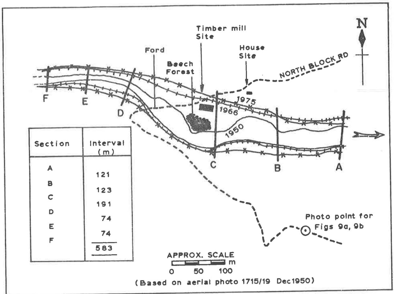
FIG 5 – Cross-sections, and active bed limits for 1950, 1966 and 1975, on McCullough's mill reach. Section intervals are for 1975.
