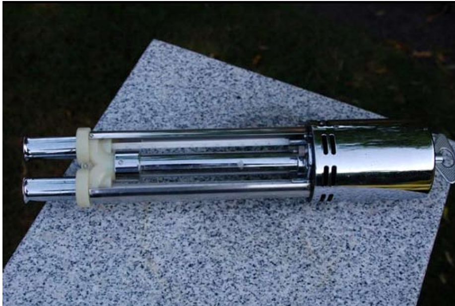
Figure 8. Portable electric fan psychrometer, with battery-powered fan and wet-and dry-bulb thermometers. Photo courtesy of British Columbia Ministry of Forests and Range, Protection Branch.
