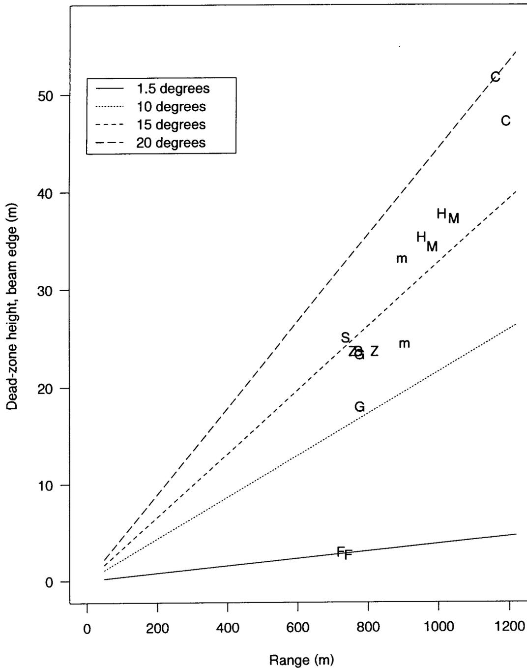
**Figure 7** Estimated average dead zone height (edge) for acoustic transects on the "flat" (F) and on the hills (C = Crypt, G = Graveyard, H = Headstone, m = Morgue, M = Mummy, S = Scroll, Z = Zombie), with reference lines for average bottom slopes from 1.5 to 20°.
