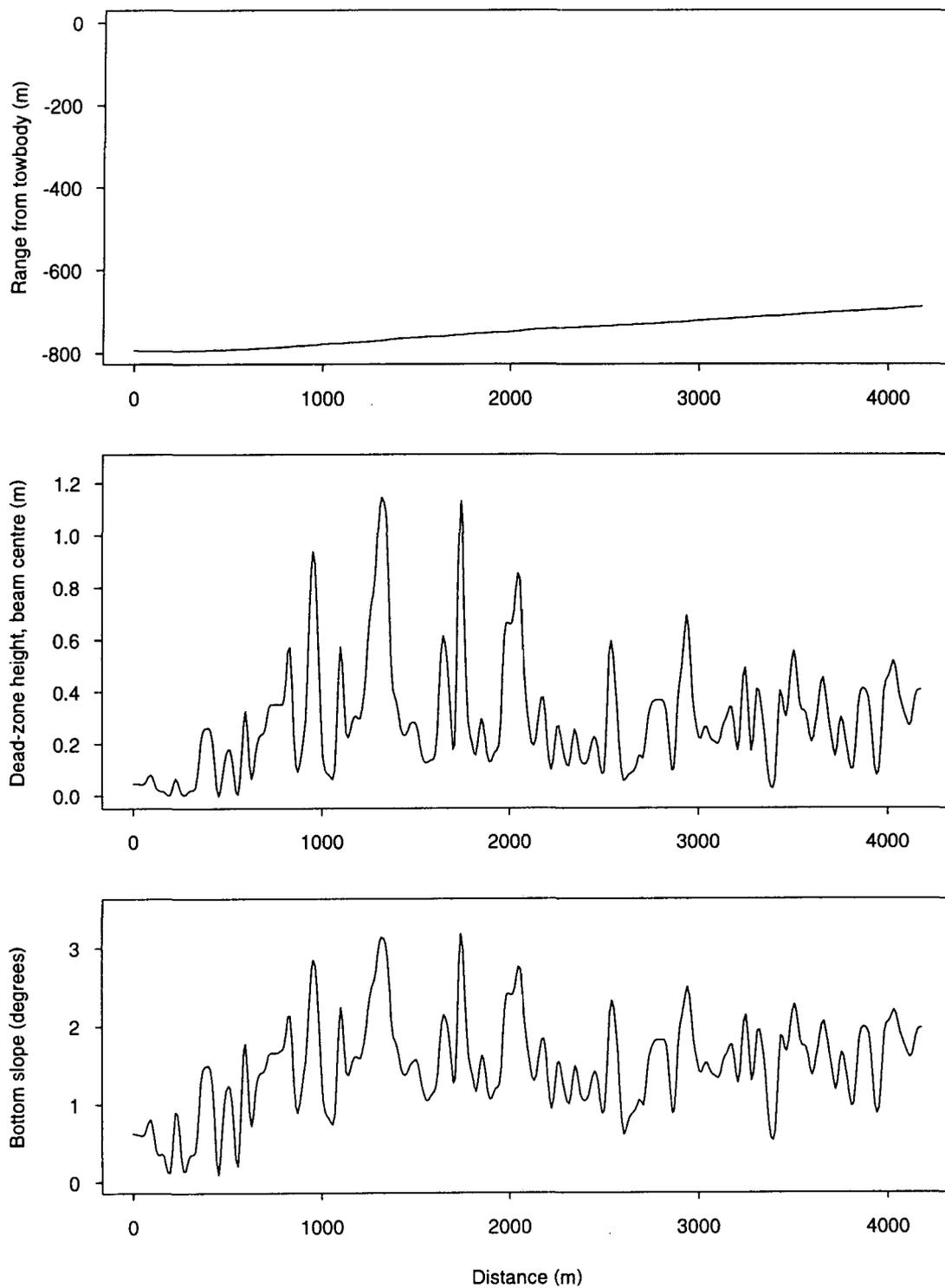
**Figure 3:** Smoothed plots for an acoustic transect recorded on the "flat": the estimated range of the bottom from the transducer; the dead zone height; and the bottom slope.
