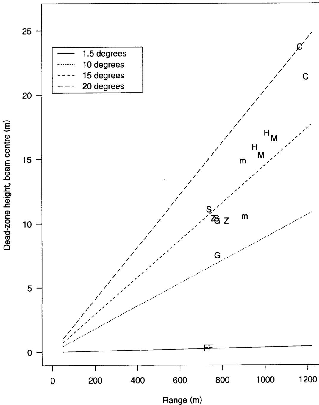
**Figure 6** Estimated average dead zone height (centre) for acoustic transects on the "flat" (F) and on the hills (C = Crypt, G = Graveyard, H = Headstone, m = Morgue, M = Mummy, S = Scroll, Z = Zombie), with reference lines for average bottom slopes from 1.5 to 20°.
