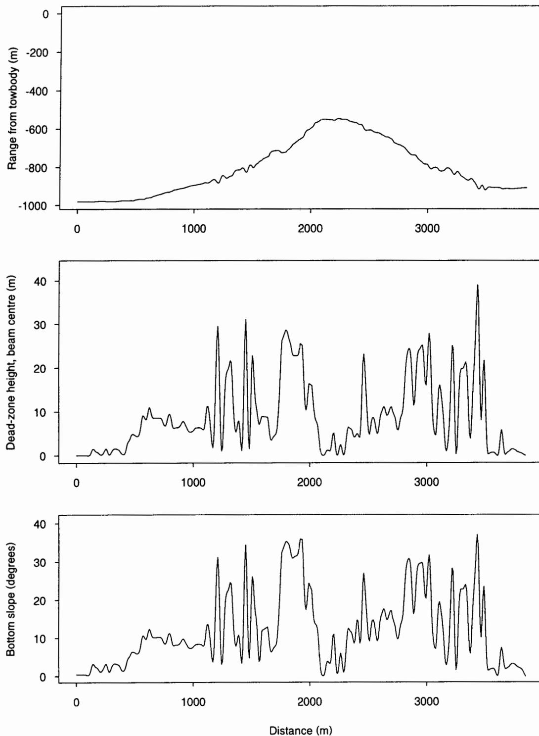
**Figure 5:** Smoothed plots for an acoustic transect recorded on the graveyard: the estimated range of the bottom from the transducer; the dead zone height; and the bottom slope.
