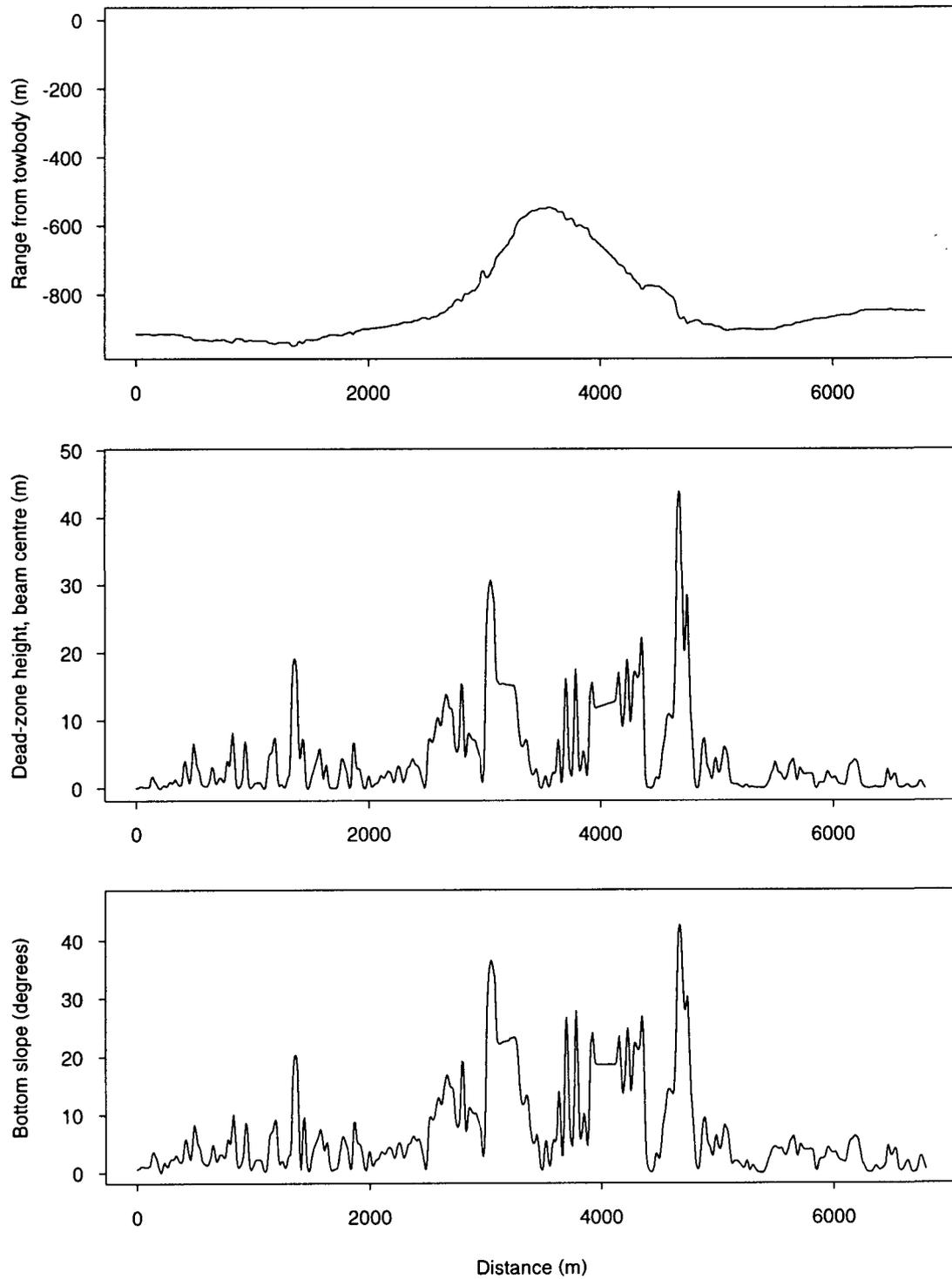
**Figure 4:** Smoothed plots for an acoustic transect recorded on the graveyard: the estimated range of the bottom from the transducer; the dead zone height; and the bottom slope.
