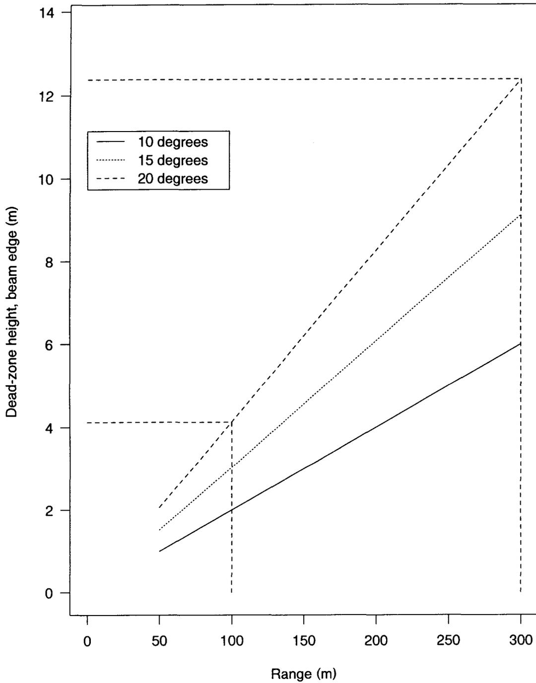
**Figure 9:** Approximate dead zone heights (edge) for hills with average slopes from 10–20° at ranges from 100 to 300 m.
