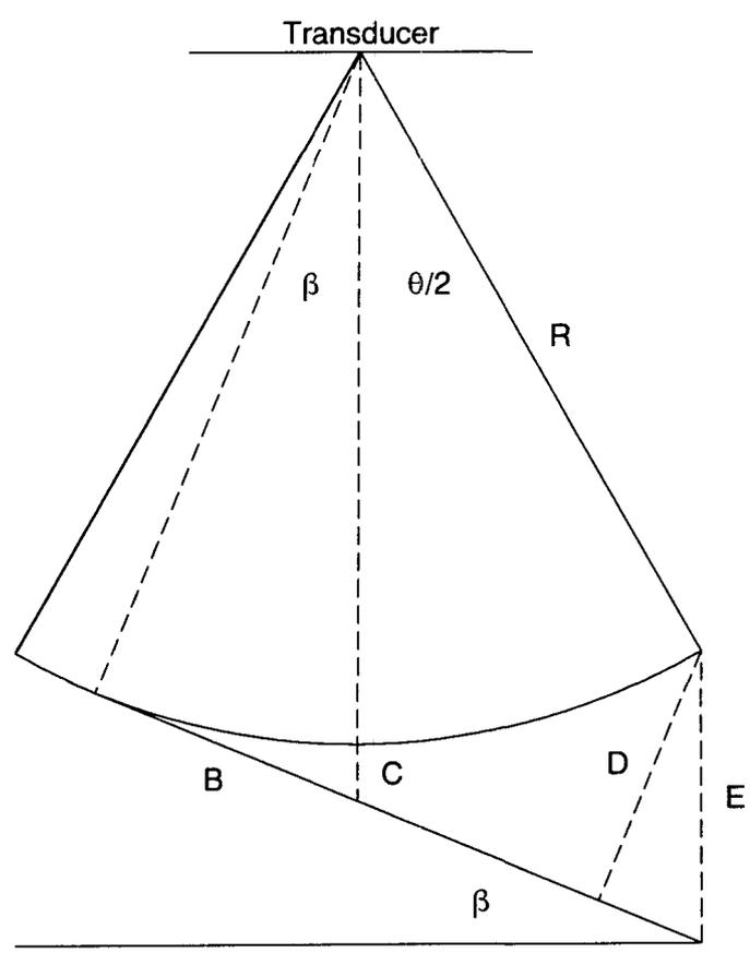
**Figure 1:** Diagram showing the definition of  $B$ ,  $C$ ,  $D$ , and  $E$  for an idealised beam (beam angle  $\theta$ ) and a sloping bottom (range  $R$ , angle  $\beta$ ). The case where  $\beta < \theta/2$  is shown.
