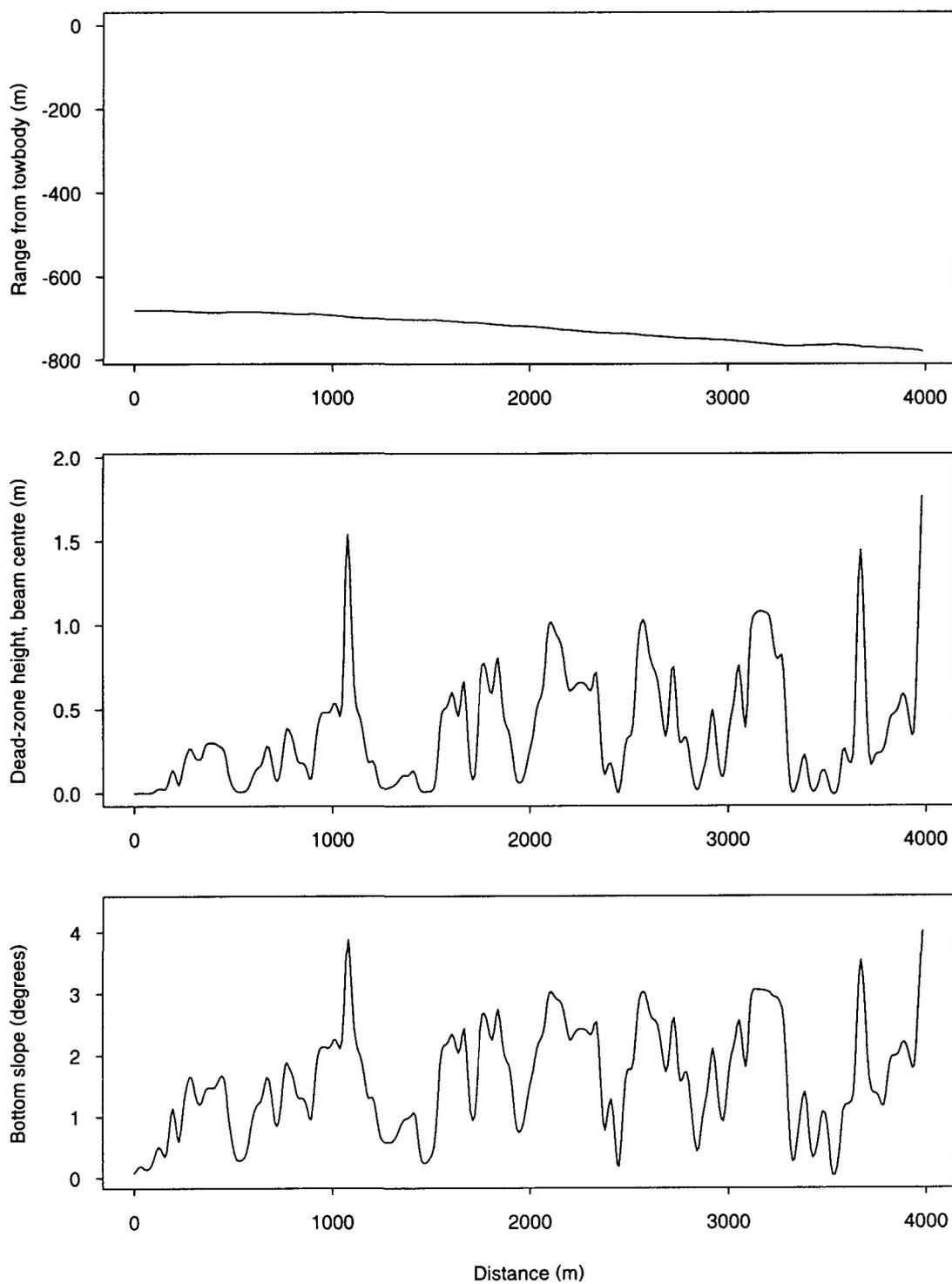
**Figure 2:** Smoothed plots for an acoustic transect recorded on the "flat": the estimated range of the bottom from the transducer; the dead zone height; and the bottom slope.
