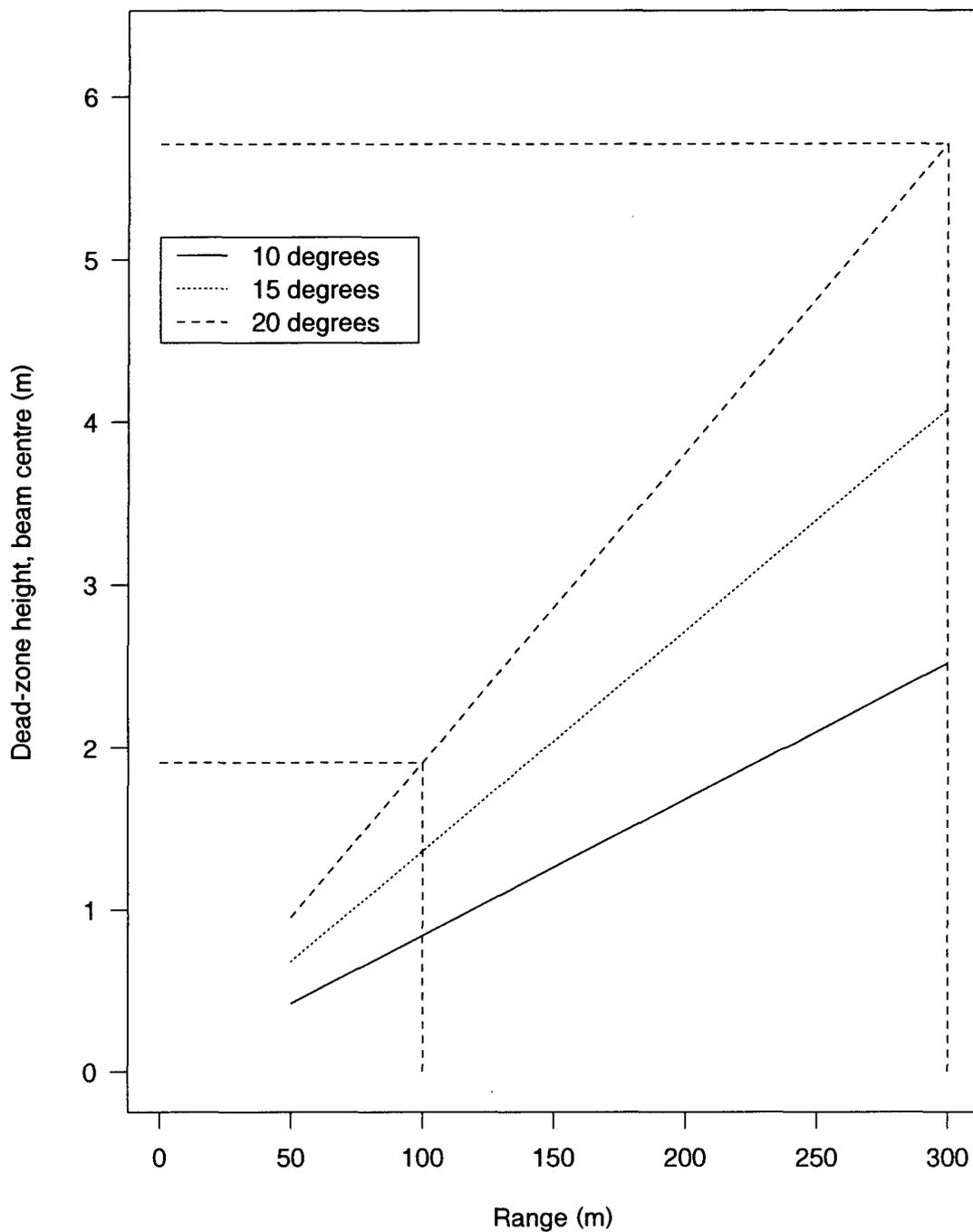
**Figure 8:** Approximate dead zone heights (centre) for hills with average slopes from 10–20° at ranges from 100 to 300 m.
