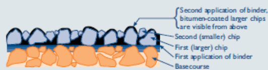
FIGURE 1.11 Two-coat seal
