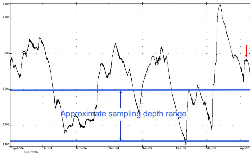
**Figure 1:** Water level record, Lake Manapouri, from September 2004 to April 2005. Red arrow indicates approximate time of sampling. Samples were taken within the depth range shown. Add 174669 to value on y-axis to obtain lake level in mm above sea level.
