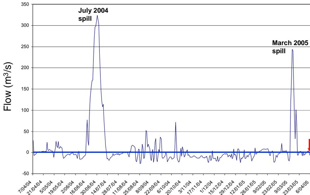
**Figure 2:** Flows in the Waiau Arm from April 2004 to April 2005, calculated as Mararoa flow – lower Waiau flow. Flows below the blue line are towards the lake and above the blue line, towards the MLC. Red arrow indicates time of survey.
