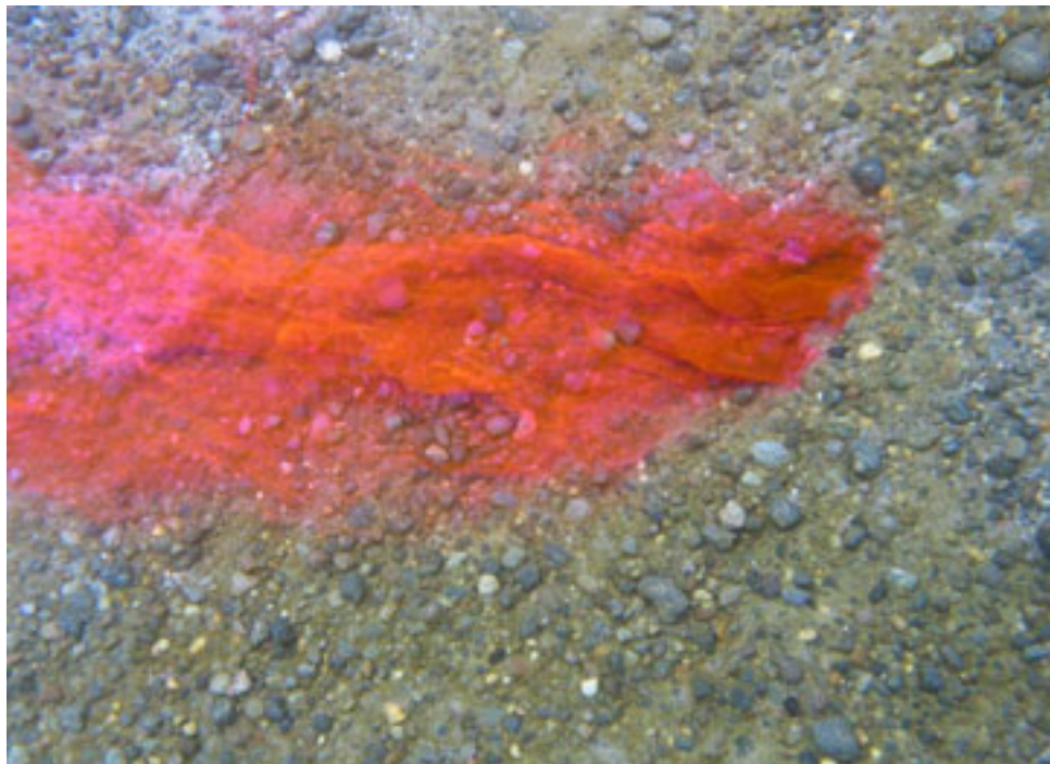
Figure 3: Dye-stained groundwater flowing from the lake bed above the point of injection.
