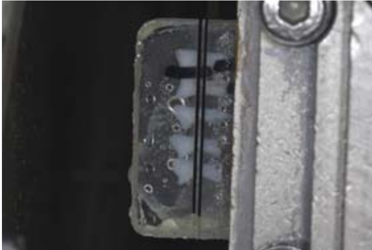
Sectioned block showing wafer still held in place by a small tag of connecting resin on the near edge.
