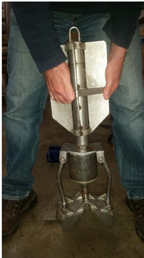
Figure 7: Clamshell grab used to collect sediment samples during the survey.
