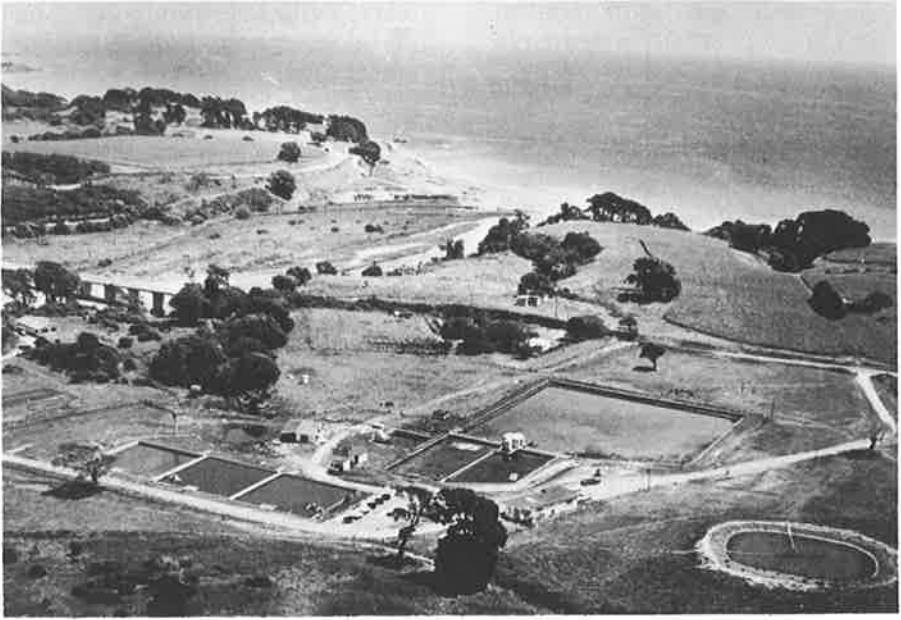
Te Kaha Aquaculture Station. Water is pumped from the river on the left to the reservoir on the extreme right. From there it siphons back to the ponds.
