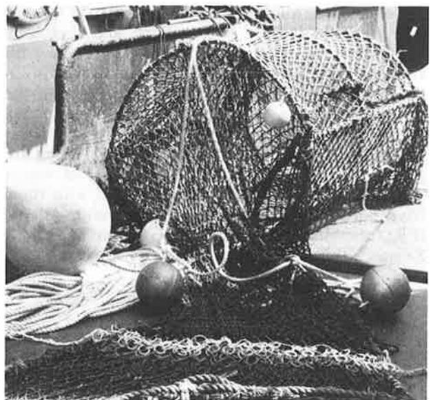
Fig. 3: Detachable cod-end for underwater tagging.
