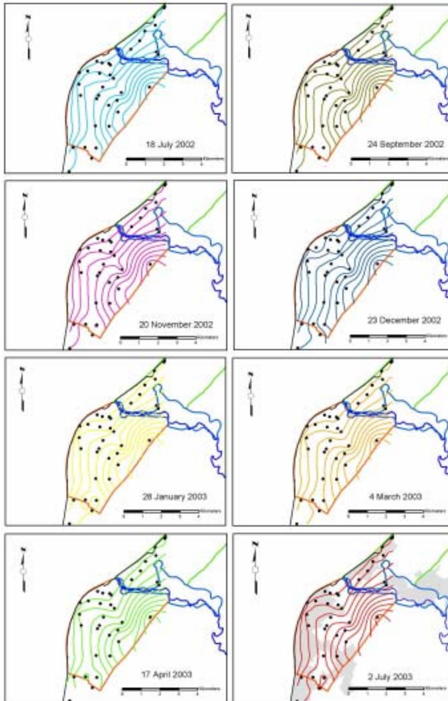
Figure 8: Water table contours for the Waikanae Groundwater Zone between July 2002 and July 2003. The contour interval is one metre with the western-most contour on each plot being one metre above mean sea level.
