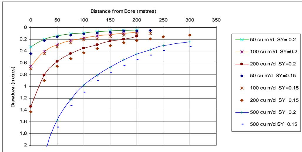
Figure 22: Modelled effects of groundwater abstraction from a single well on wetland water levels at a variety of pumping rates
