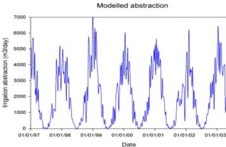
Figure 14: Calculated cumulative irrigation abstraction from the shallow sand aquifers on the Kapiti Coast
