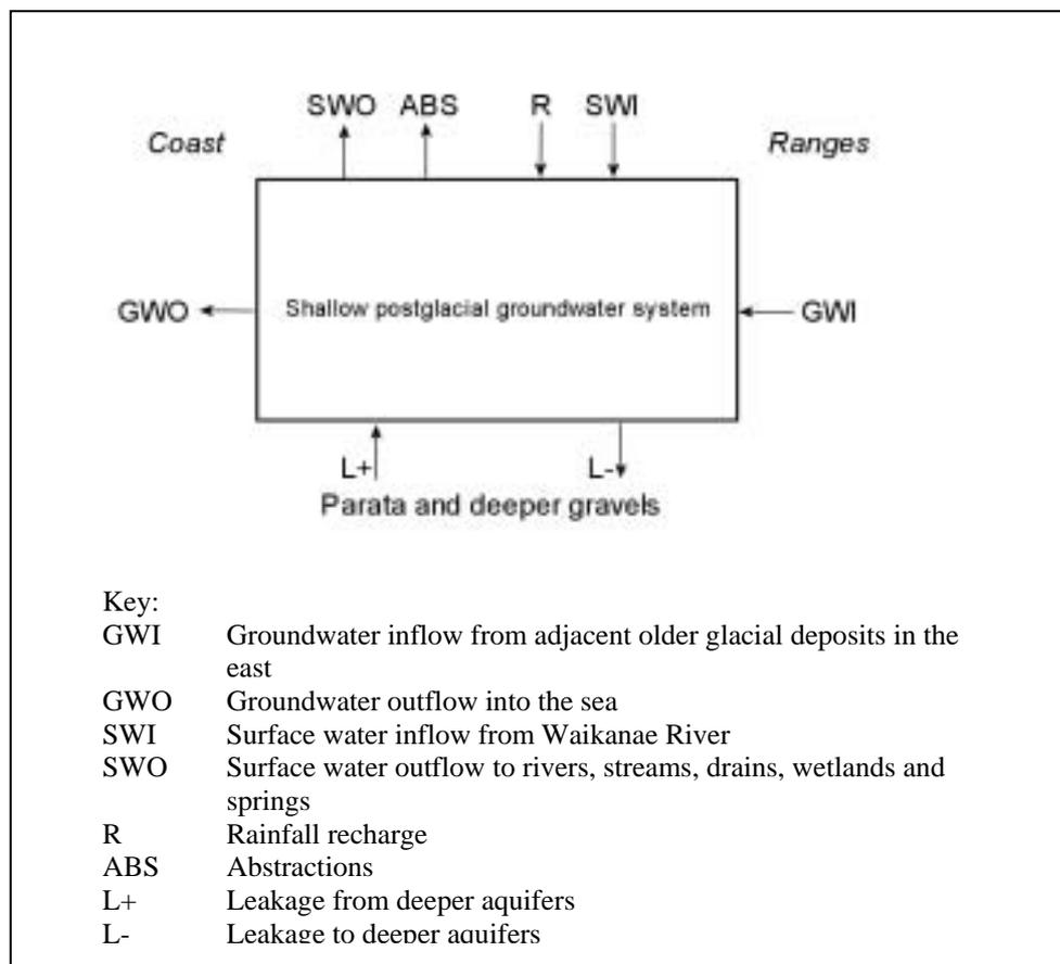
Figure 15: Conceptual Groundwater Balance – Kapiti Unconfined Aquifers
