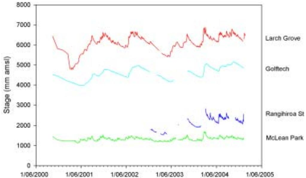
Figure 6: Waikanae Groundwater Zone monitoring well hydrographs
