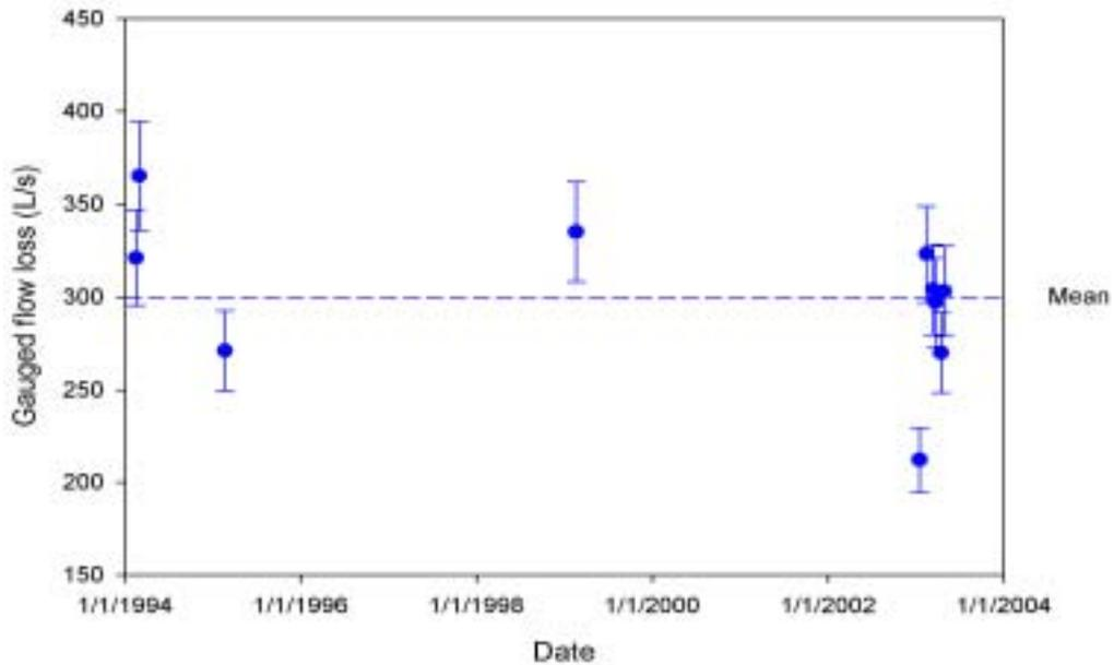
Figure 12: Waikanae River gauged flow losses between SH1 and Jim Cooke Park. The error bars show +/-8%
