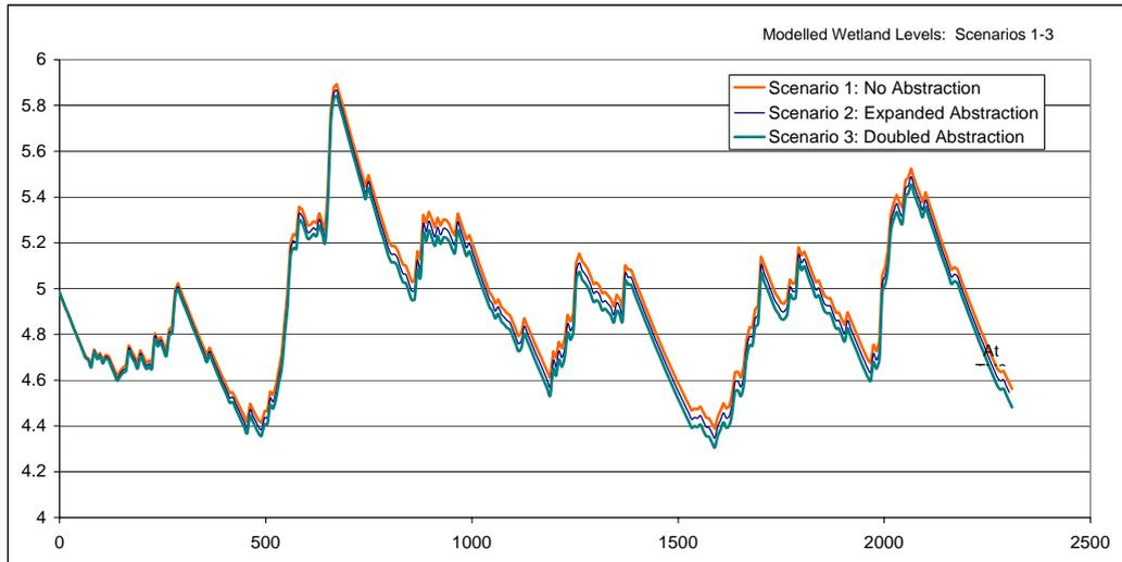
**Figure 21: Modelled effects of shallow groundwater abstraction on water level in the Te Harakeke Wetland (no abstraction, current/expanded abstraction and twice current abstraction)**
