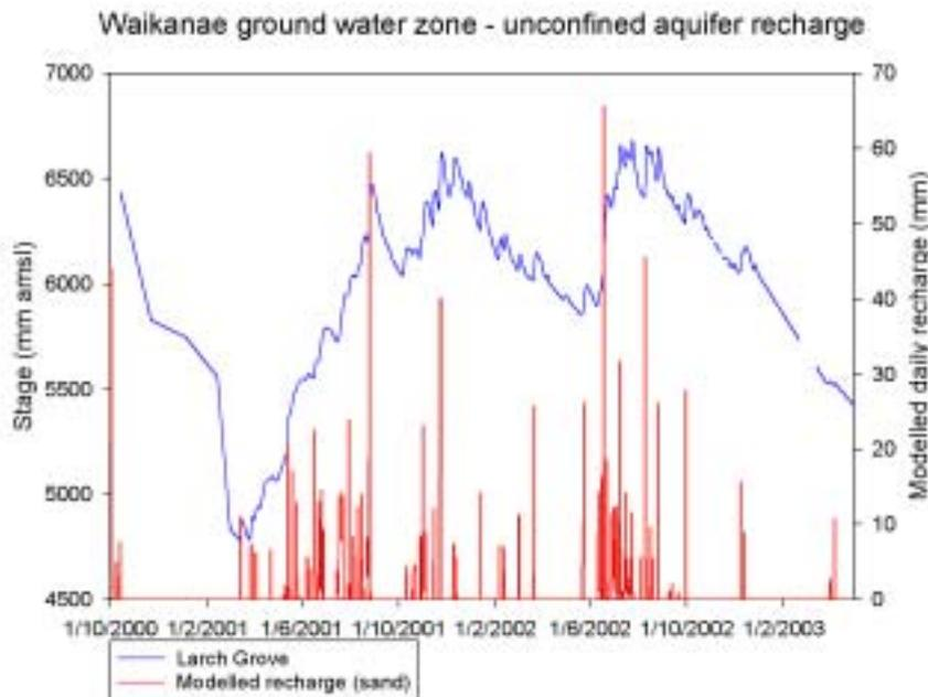
Figure 7: Calculated groundwater recharge and observed groundwater level in the Larch Grove monitoring well
