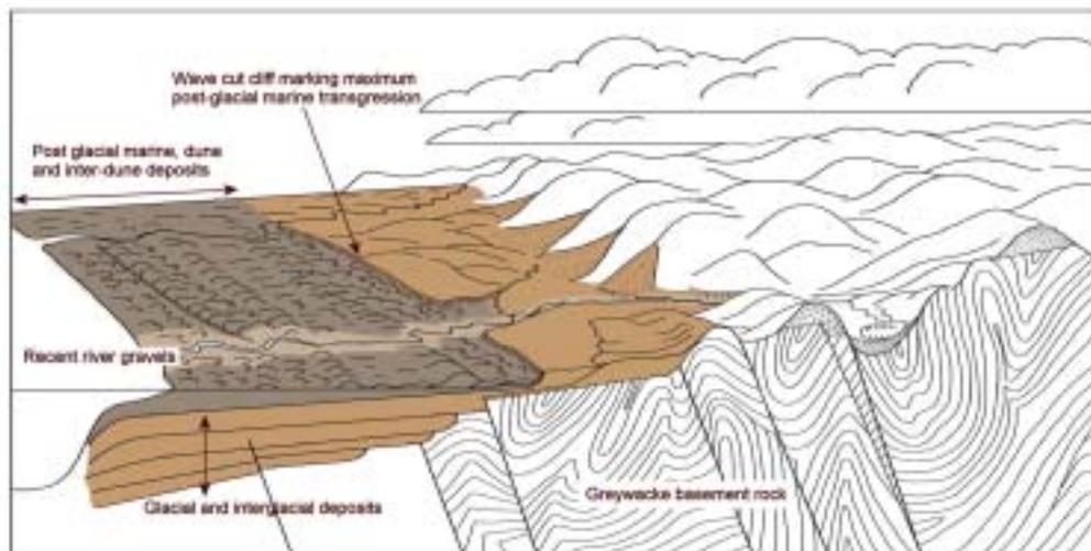
Figure 2: Diagrammatic cross section through the Waikanae area to illustrate the local geological succession
