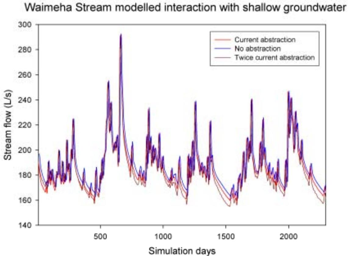
Figure 20: Modelled effects of shallow groundwater abstraction on flows in the Waimeha Stream (no abstraction, current abstraction and twice current abstraction)
