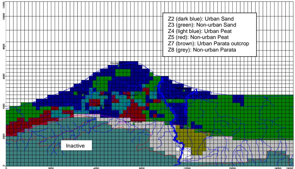
Figure 18: Recharge zones based on soil type and urban area
