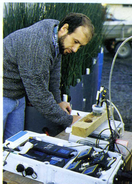
Measuring physiochemical conditions in the root zone of wetland microcosms.
