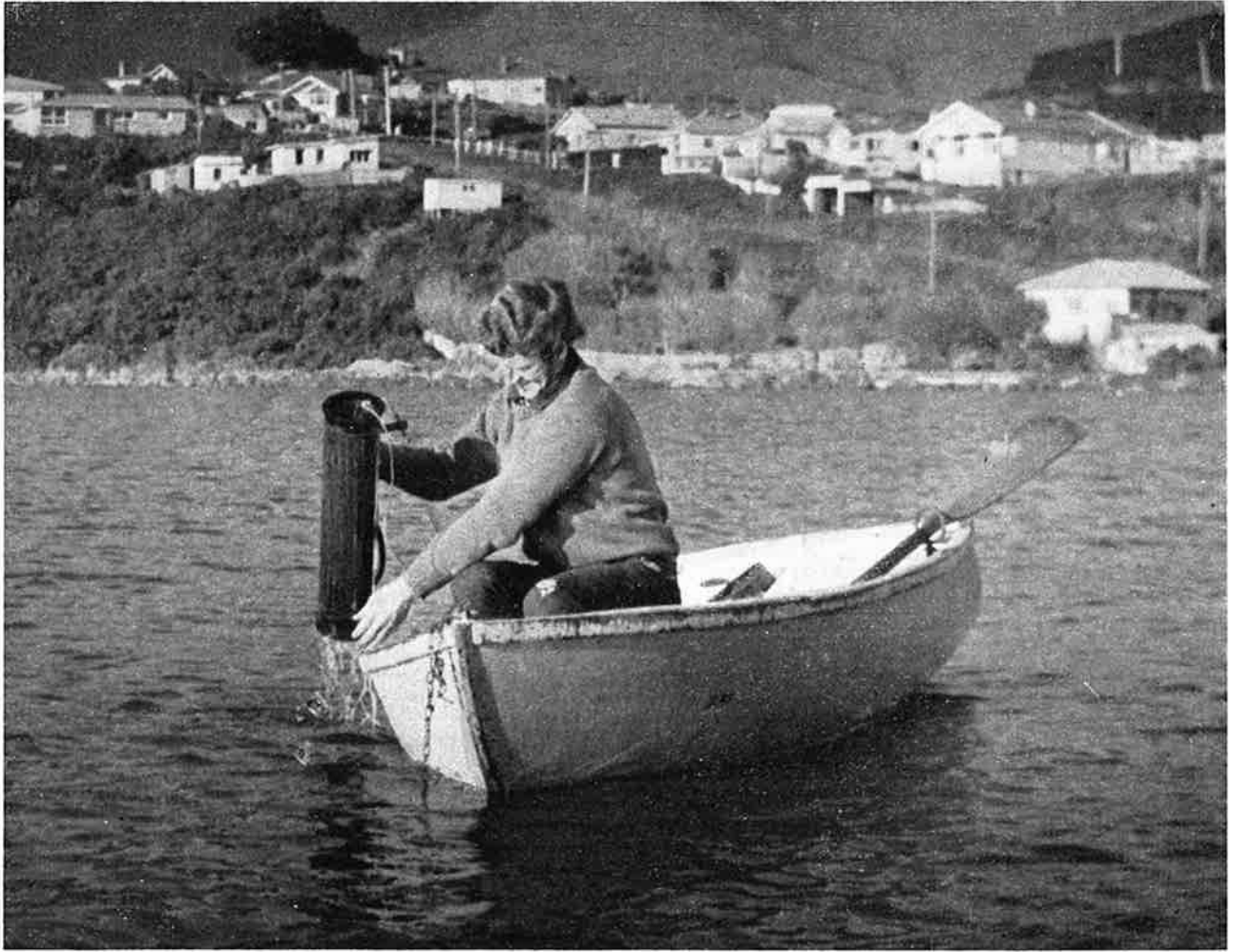
Frontispiece: Water samples being taken from Tomahawk Lagoon with a Van Dorn sampler on a calm winter's day.
