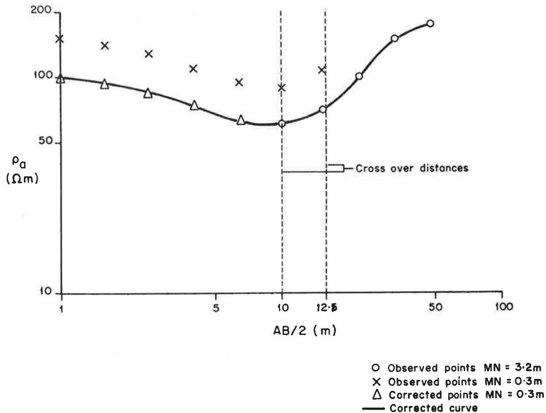
Fig. 2: Illustration of the effect of curve smoothing. In this example, observed resistivities with an  $MN$  of 0.3 m were corrected to give the final curve.
