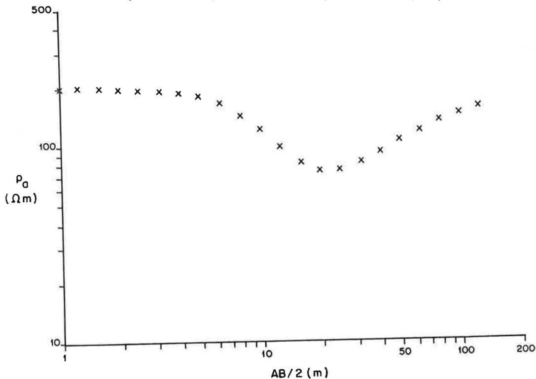
Fig. 8: A three layer sounding curve.
