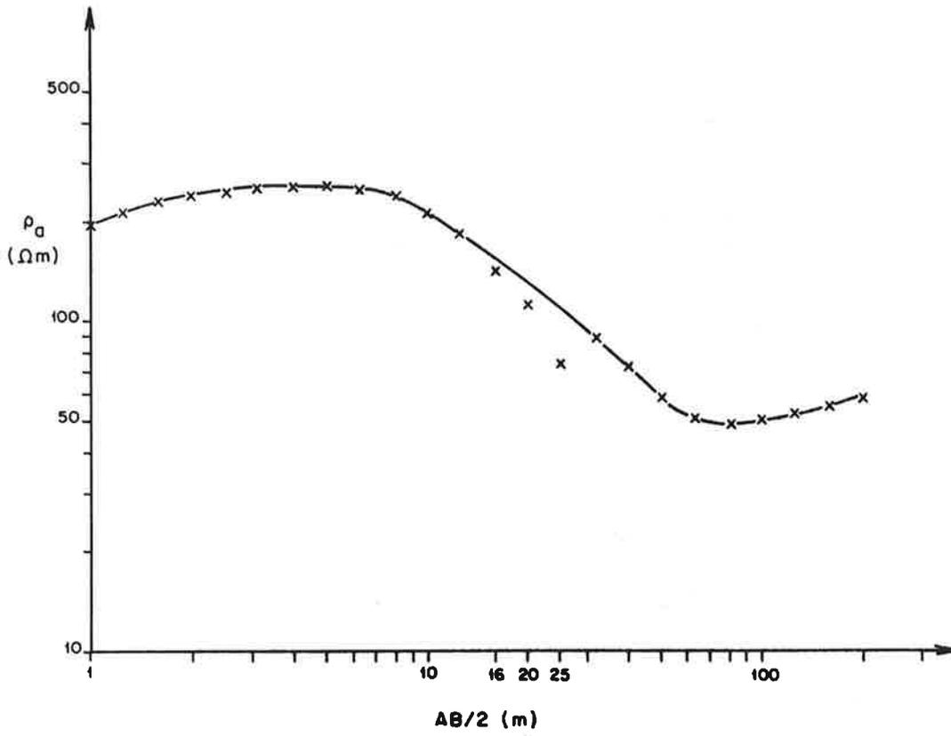
Fig. 4: A sounding curve showing effects of a lateral resistivity variation. Data at  $AB/2 = 16, 20$  and  $25$  m are affected by the lateral change and are ignored when drawing the 'corrected' curve.
