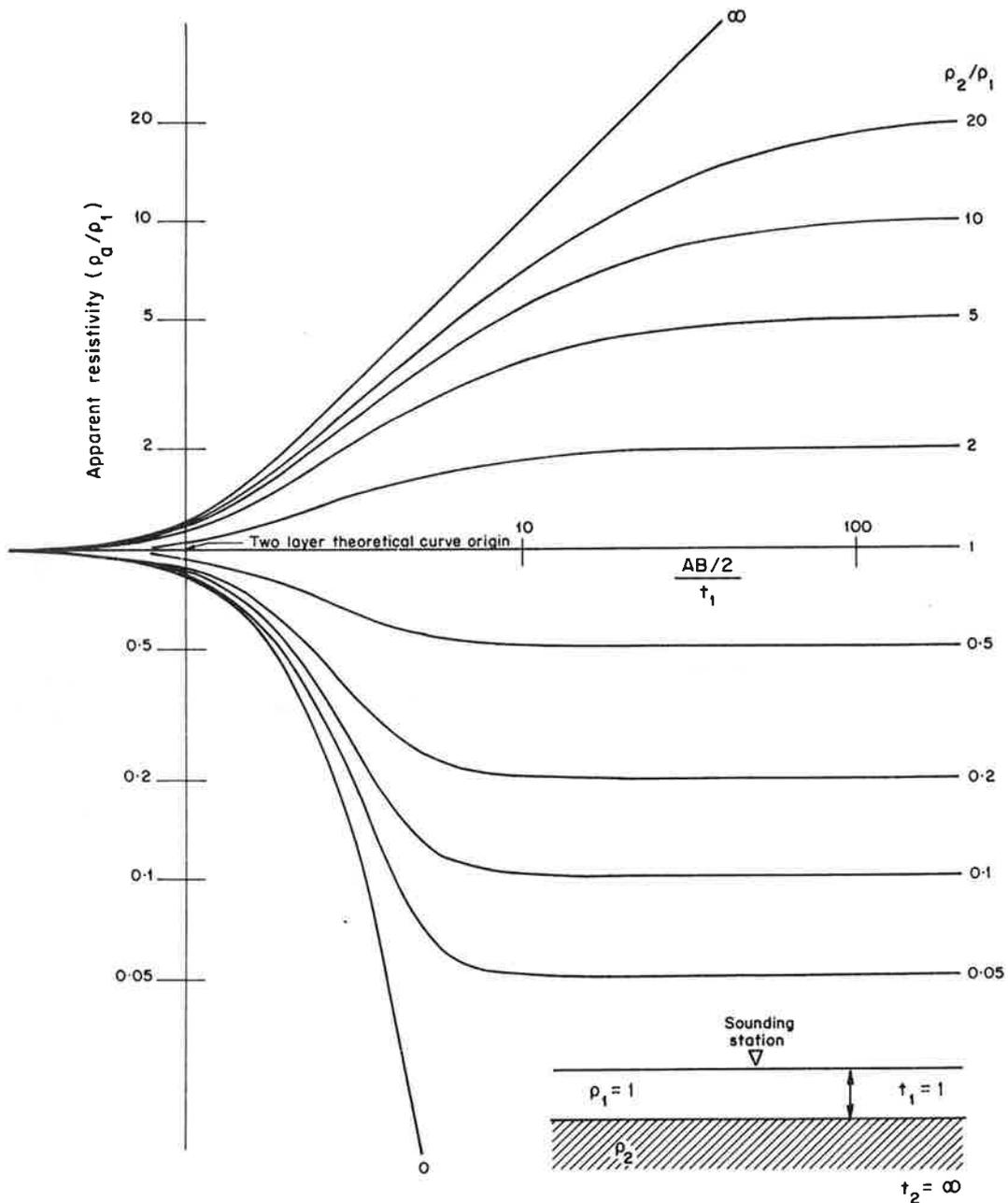
Fig. 6: Theoretical two layer sounding curves for the Schlumberger array (after Orellana and Mooney, 1966).
