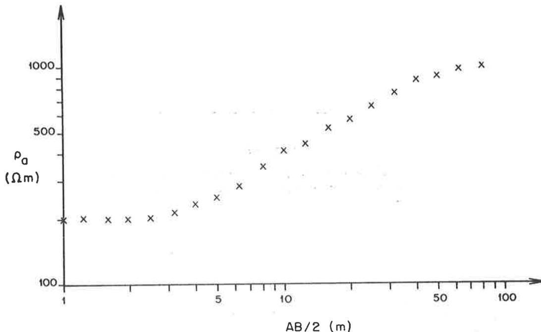
**Fig. 3:** Sounding curve of corrected resistivity data from Table 2.
