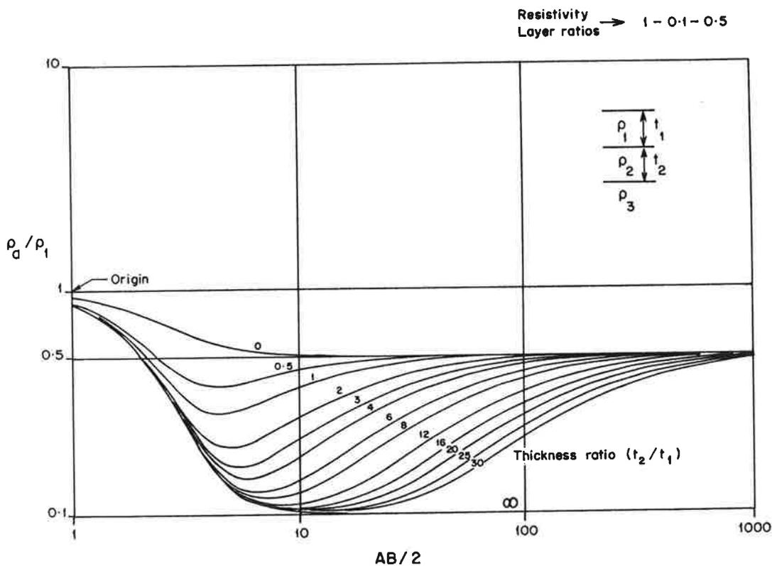
Fig. 9: A group of standard three layer curves for the Schlumberger array (after van Dam and Meulenkamp, 1969).
