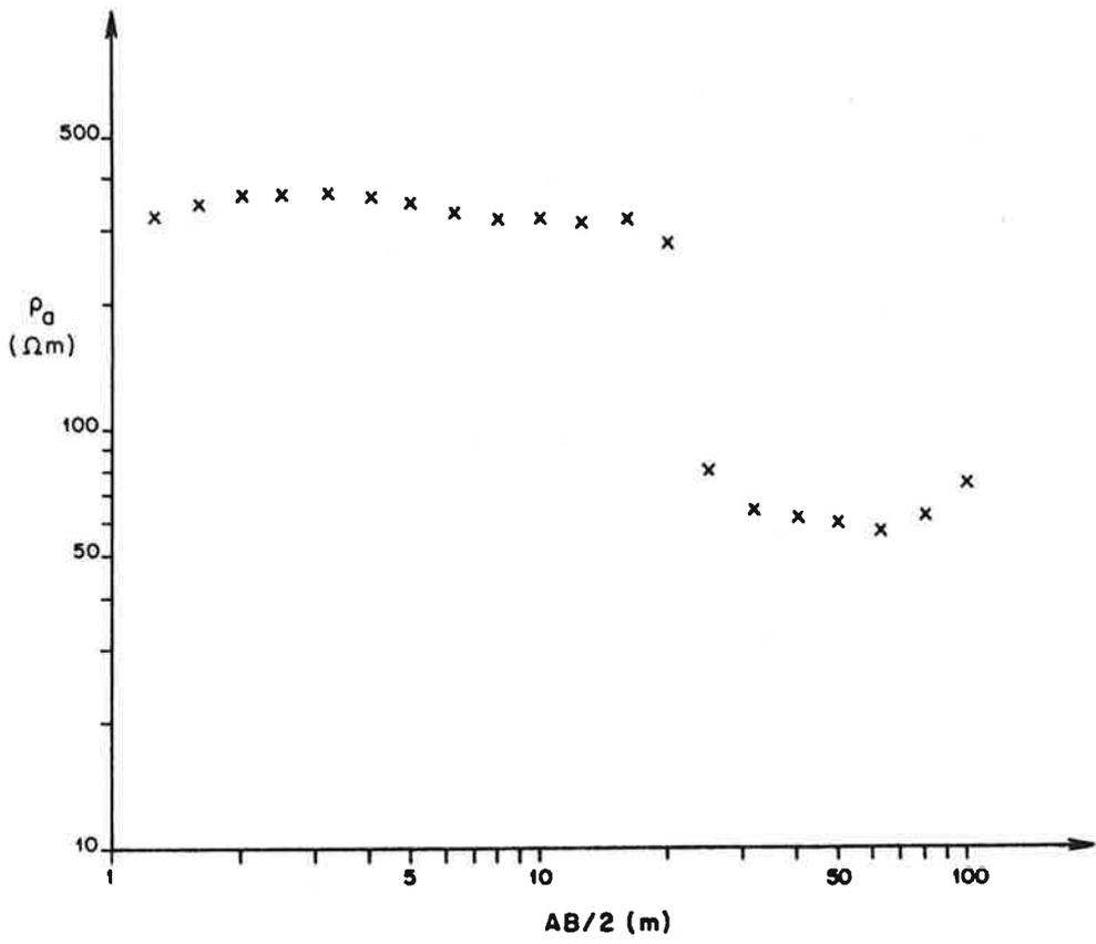
Fig. 5: Sounding curve affected by large scale lateral resistivity variation. This curve is not interpretable purely in terms of resistivity varying with depth under the sounding site.
