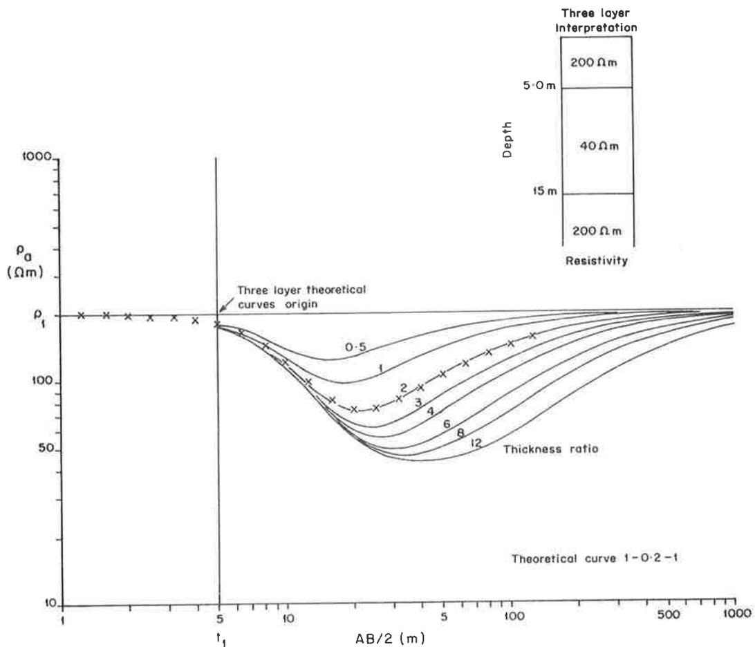
**Fig. 10:** Illustration of a three layer interpretation by curve matching. The crosses are the field observations. The geo-electric section of the best fit theoretical curve is shown.
