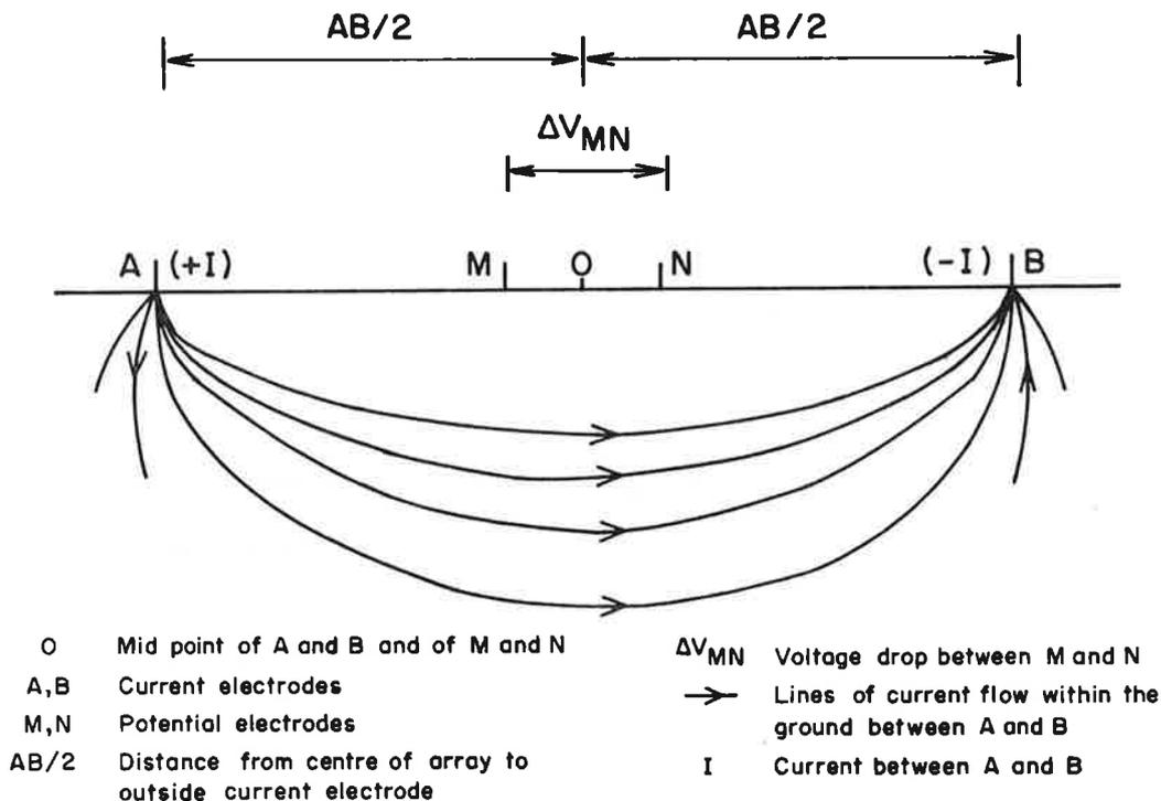
Fig. 1: Schlumberger electrode array and schematic current distribution within the ground.
