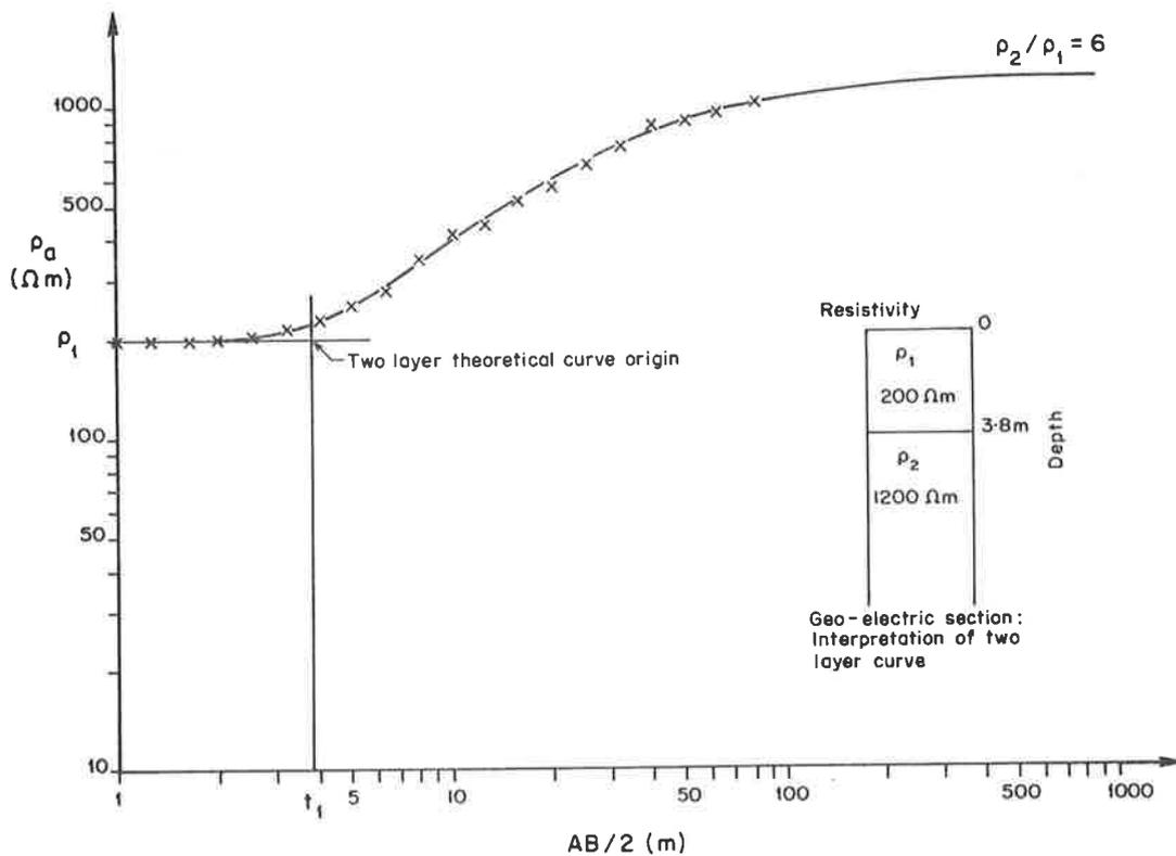
Fig. 7: The field curve of Fig. 3 (crosses) matched to a theoretical two layer curve (solid line) and resulting geo-electric section.
